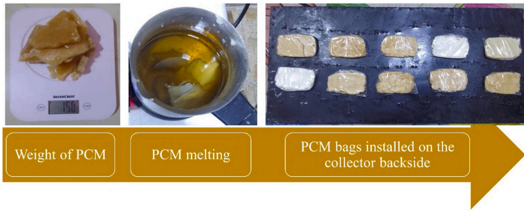
Fig. 3. Preparation procedure of PCM thermal bags.
