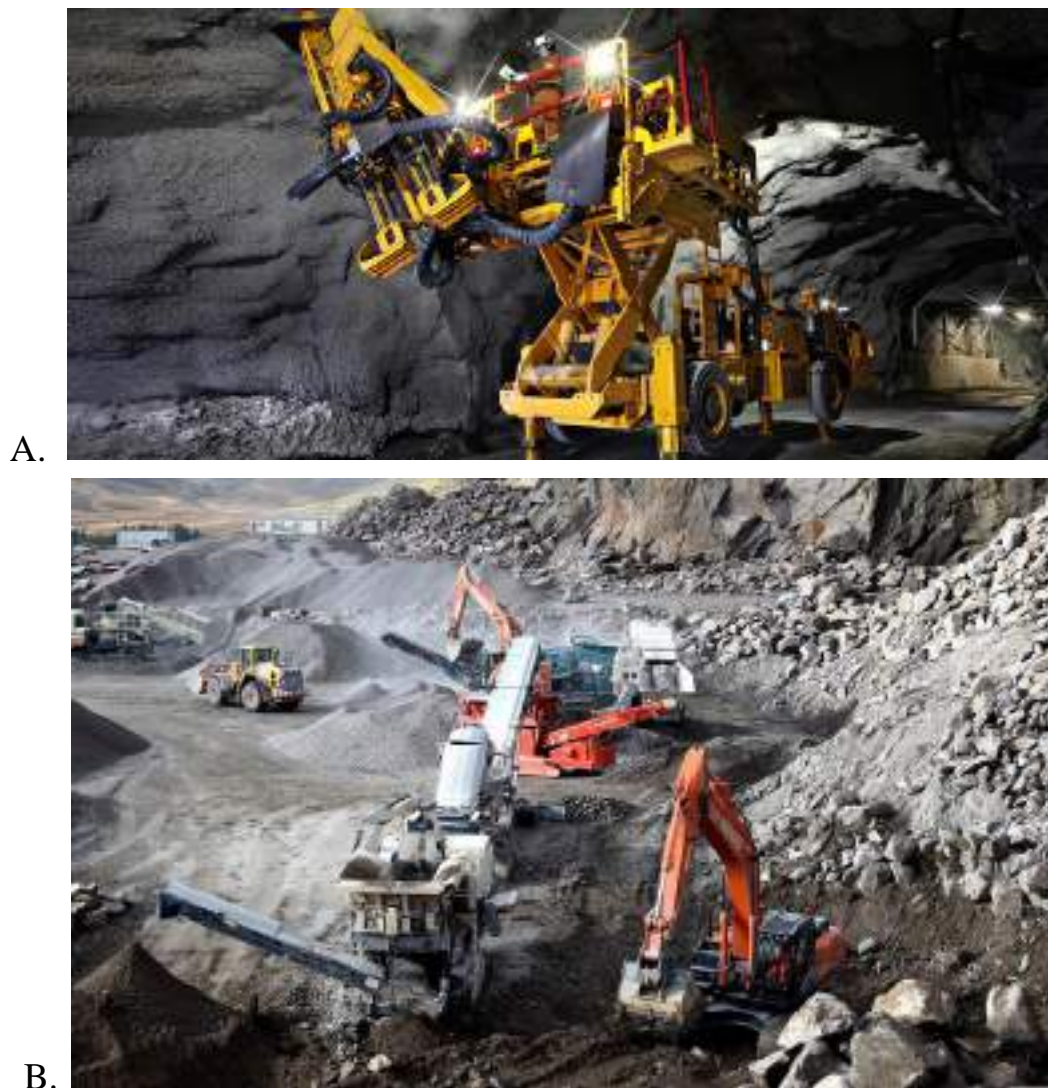
Fig.5.20 The two main type of quarries, A. Subsurface quarry or mine Surface mine or open pit.
