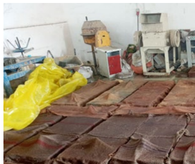
Fig.3: Casting, curing procedure, and slab specimens.
