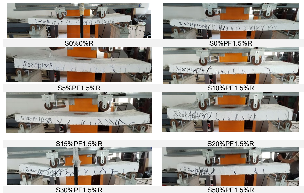
Fig.16: The crack pattern for all slabs.
