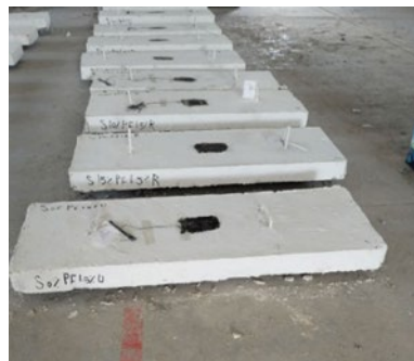
Fig.3: Casting, curing procedure, and slab specimens.
