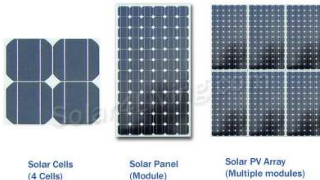
Figure 3.4. The configuration of a PV array [106]
