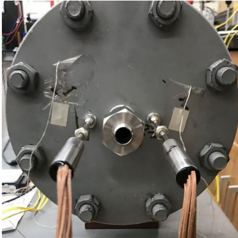
Figure B3: Cover Flange (inlet side) which was used to study the charging process with radial flow configuration.
