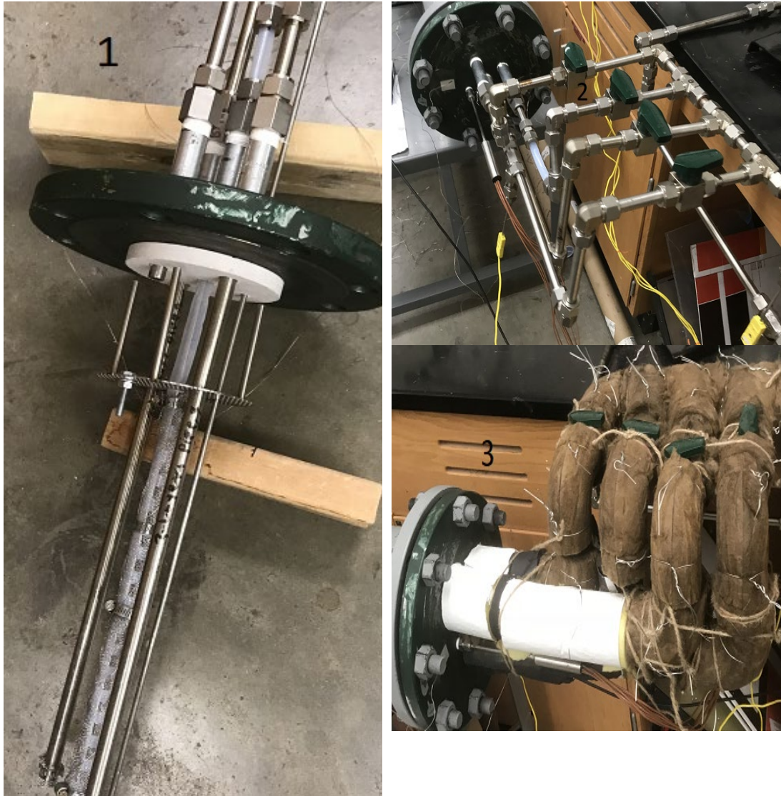
Figure B2. Custom flange for pipe injection showing the injected pipes with perforated plate as one piece. The flow in the injected pipes was controlled using several valves. Note: Image 1 shows inserting of a radial tube (primarily radial testing). However, for pipe injection, the same procedure was used.
