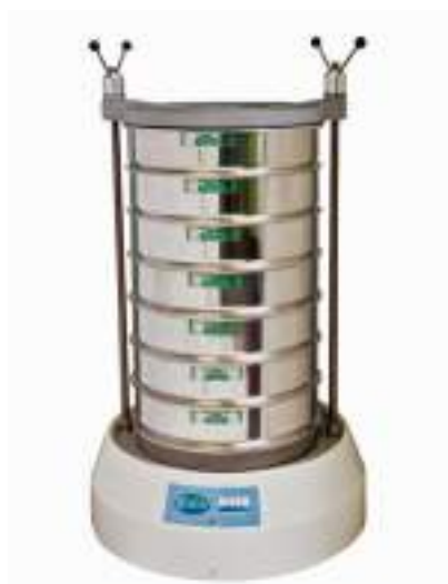
Figure 3-12 Mechanical sieves shaker
