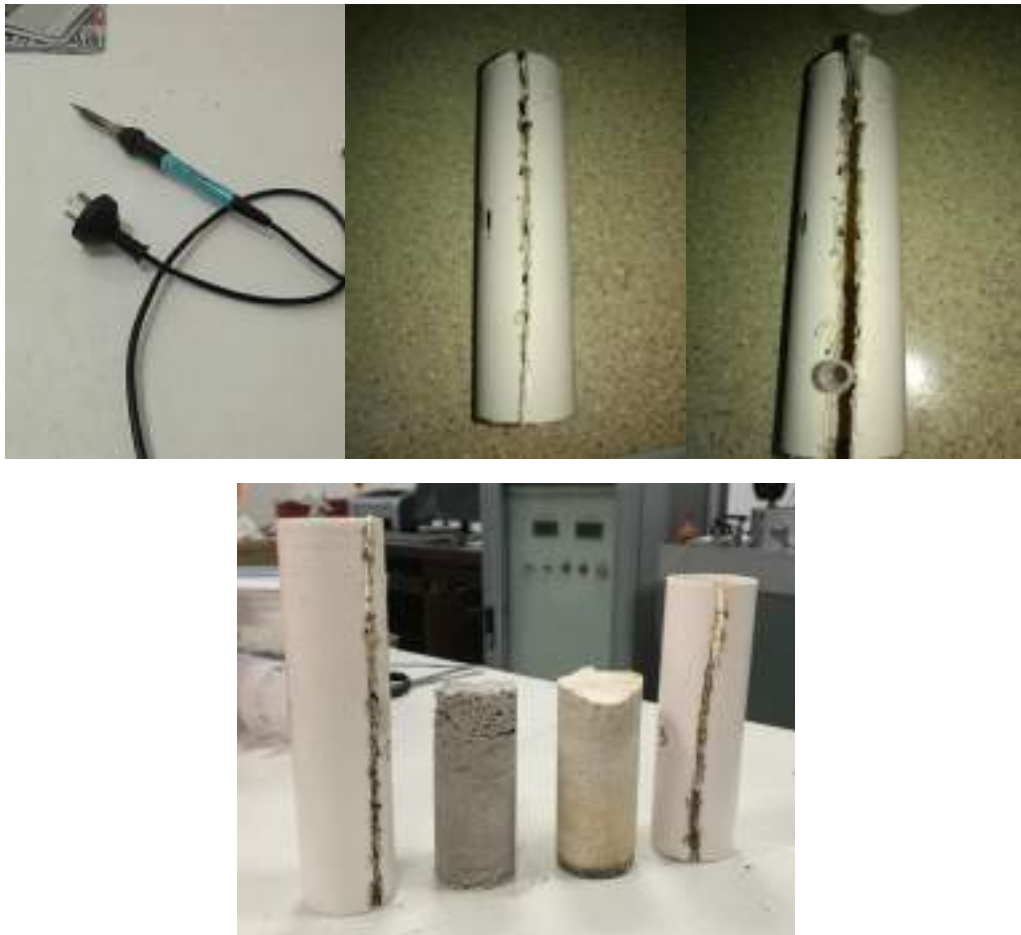
Figure 3-14 Taking out soil specimen from the PVC column
