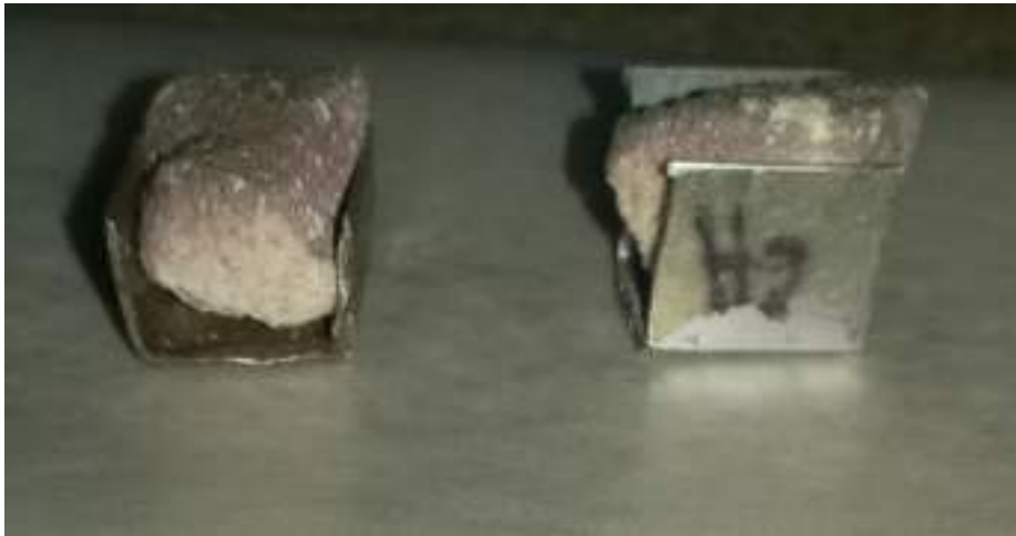
Figure 3-21 The sample used with SEM test after coated with gold
