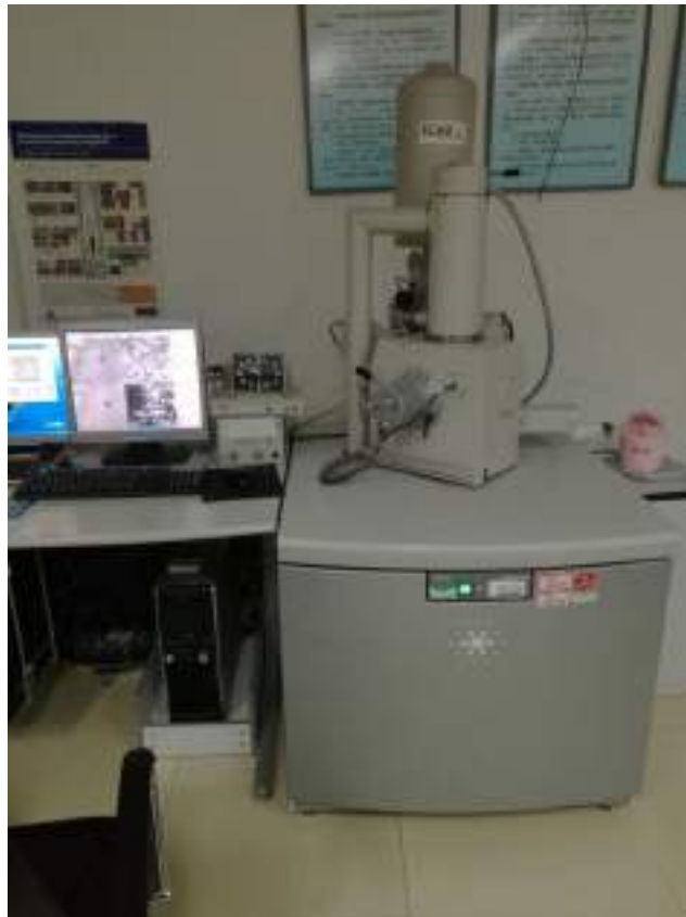
Figure 3-22 FEI Quanta 200 ESEM/VPSEM scanning electron microscope
