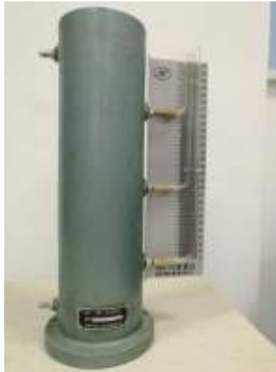
Figure 3-19 TST-70 permeameter (Constant Head Test device)
