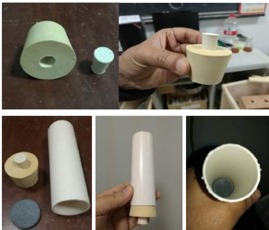
Figure 3-13 Preparation of the PVC column
