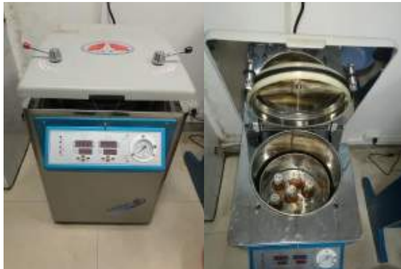
Figure 3-4 Autoclave device and nutrient broth after the end of sterilization process
