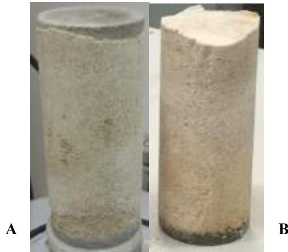
Figure 5-1 The soil samples after treatment A. Yangtze river sand B. Silica sand
