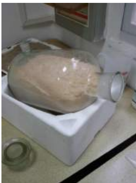
Figure 3-8 Egg shells reaction with the hydrochloric acid inside the glass reactor
