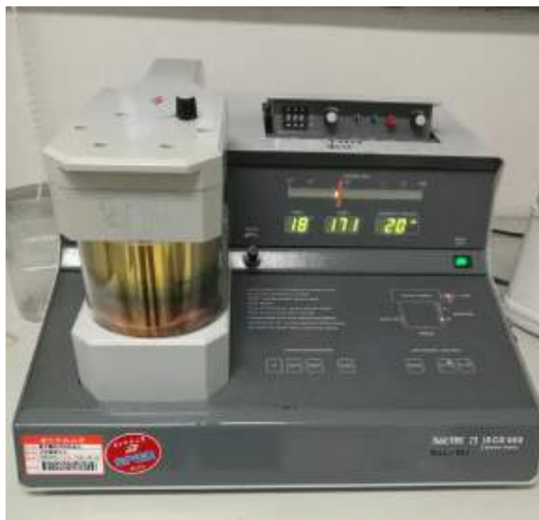
Figure 3-23 BAL-TEC / SCD 050 sputter coater
