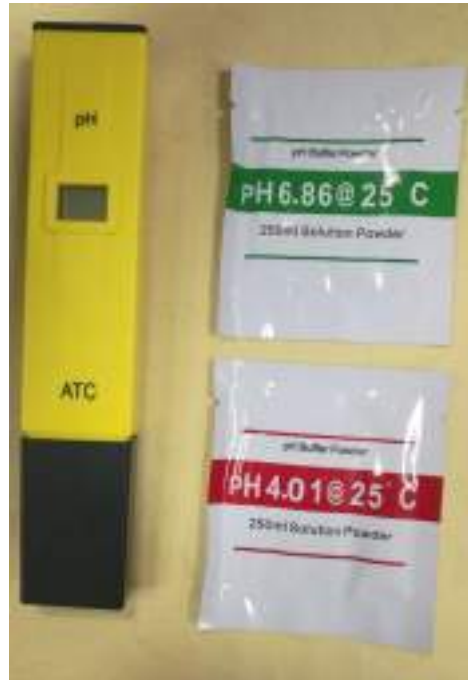
Figure 3-18 Pen type pH meter
