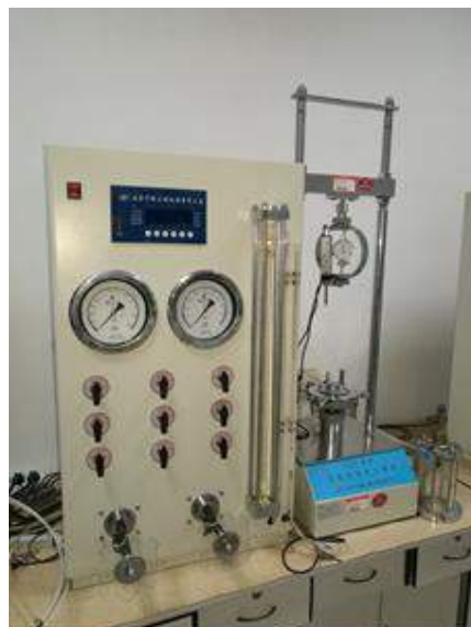
Figure 3-16 TSZ-3 machine to conduct unconfined compressive strength
