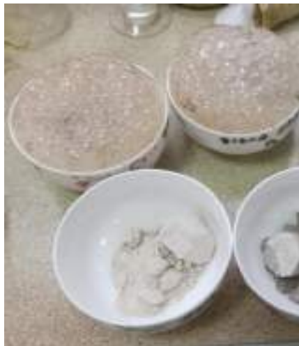
Figure 3-20 The samples soaked in hydrochloric acid
