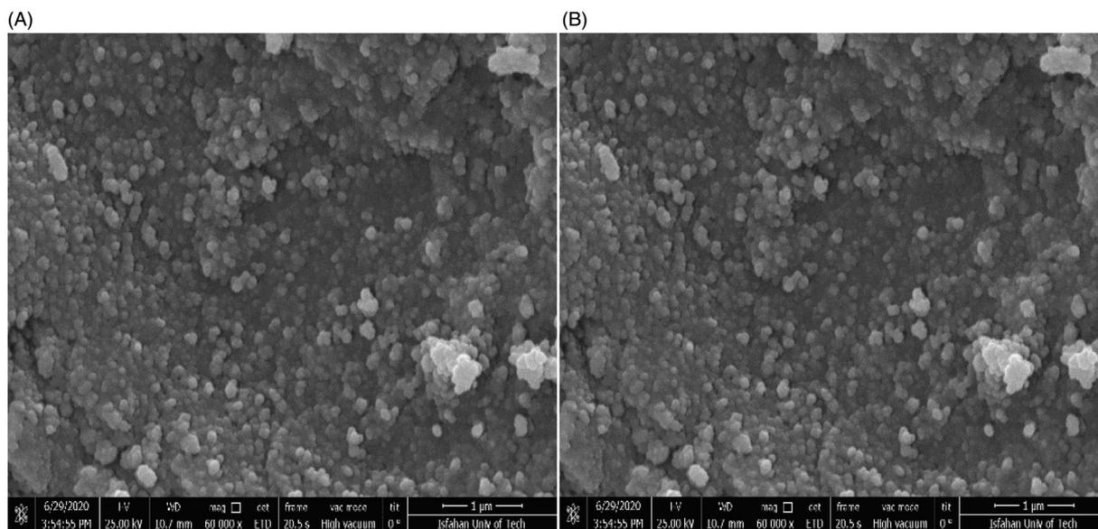
**Figure 1.** FESEM images of prepared TiO<sub>2</sub> NPs with different magnification (A and B). Abbreviations: FESEM, Field emission scanning electron microscope; TiO<sub>2</sub>, titanium dioxide. NPs, Nanoparticles.
