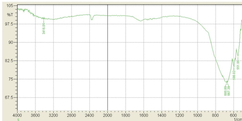
**Figure 5.** FTIR spectrum of anatase TiO<sub>2</sub> nanoparticles indicating relative functional groups.
