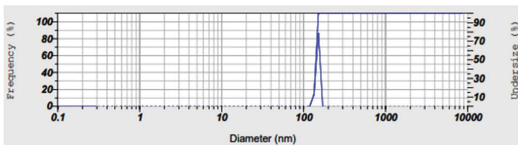
**Figure 3.** Dynamic light scattering (DLS) image of titanium nanoparticles size  $\text{TiO}_2$  NPs distribution by volume of particles (DLS) using HORIBA Scientific Nanoparticle analyzer SZ-100.
