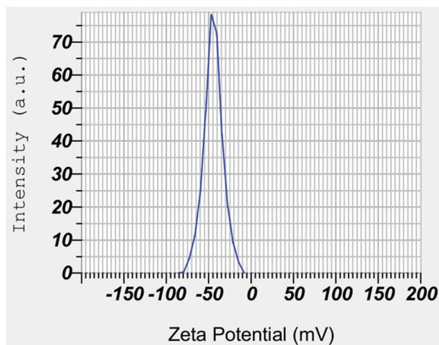
**Figure 4.** Zeta potential analysis of prepared  $\text{TiO}_2$  nanoparticles.
