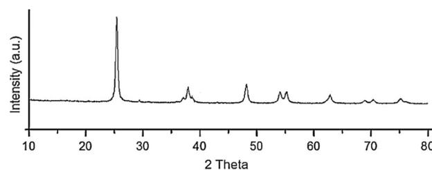
**Figure 2.** XRD pattern of prepared TiO<sub>2</sub> NPs by the sol-gel method. Abbreviations: XRD, X-ray diffraction; TiO<sub>2</sub>, titanium dioxide; NPs, Nanoparticles
