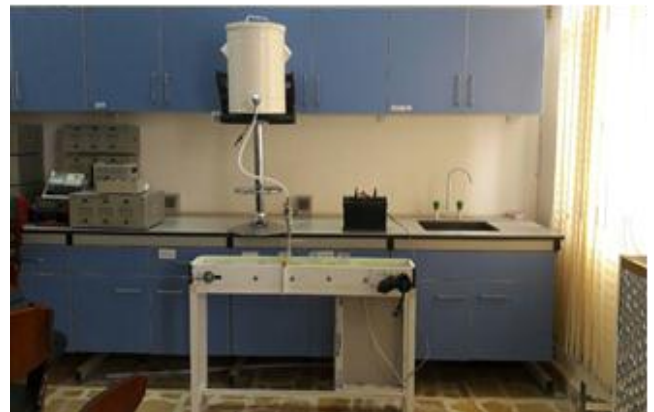
Fig-10: The overall water filling system.
