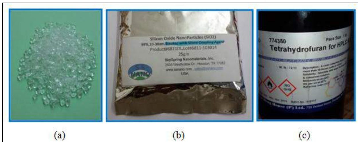
Figure (4-2) (a) PMMA granules, (b) Silicon oxide nanoparticles (SiO 2 ) and (c) Tetrahydrofuran solvent.
