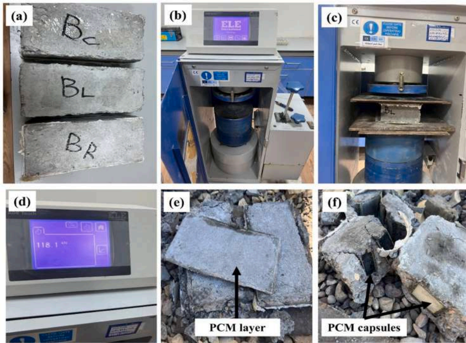
Fig. 11. Compression test (a) brick samples, (b) test machine, (c) B_L under test, (d) display monitor, (e) B_L after test, (f) B_C after test.
