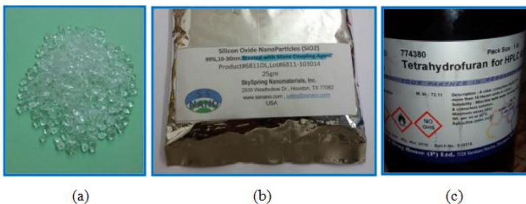
Fig.1. (a) PMMA granules, (b) Silicon oxide nanoparticles ( \text{SiO}_2 ) and (c) Tetrahydrofuran solvent
