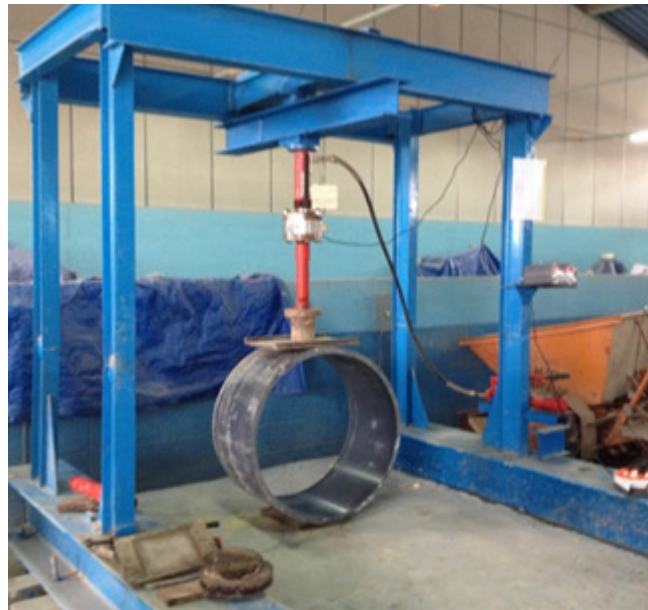
Fig. (3): Parallel Plate Loading Test
