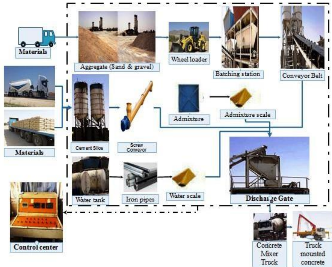
Fig. 14. Flow of process in the production of ready mix concrete ( Researcher ).
