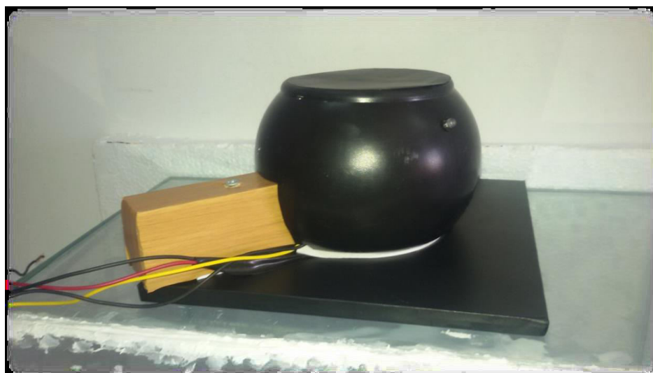
Figure 12): Final design of the piezoelectric generator
