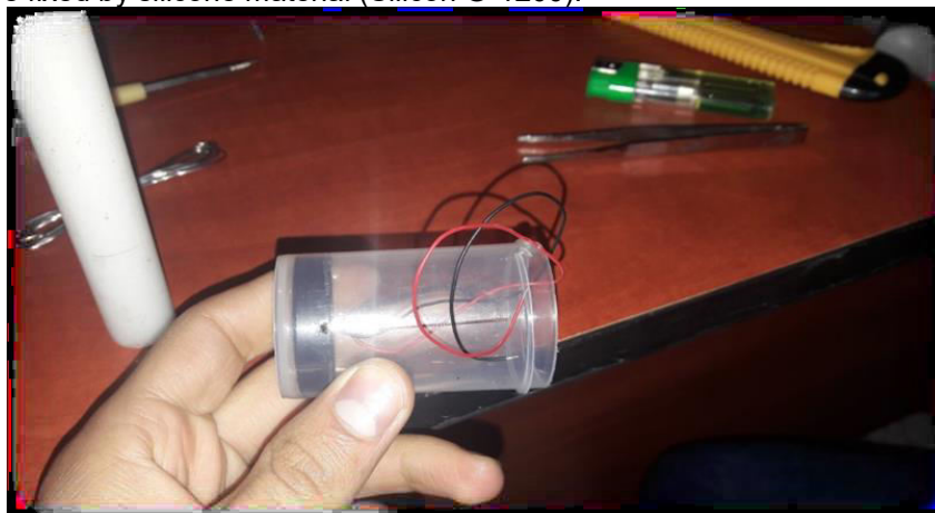
Figure 14: The piezoelectric cell fixed at the end of the tube
