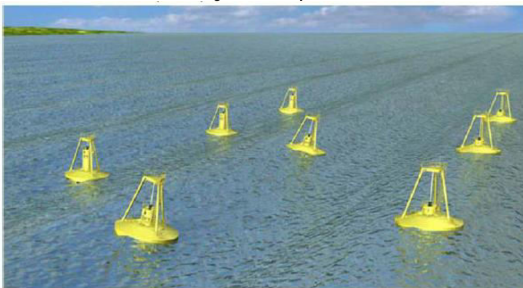
Figure 8: A field of point absorber (OPT) devices.
