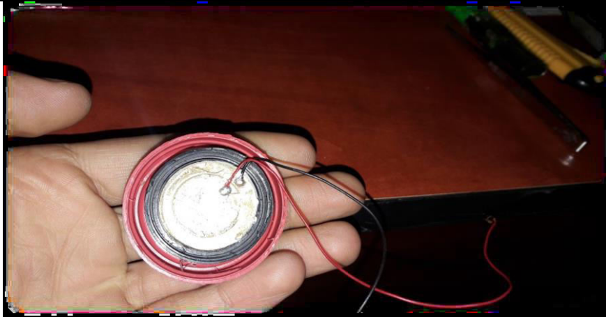
Figure 15: Piezoelectric cell fixed on the cap of the tube
