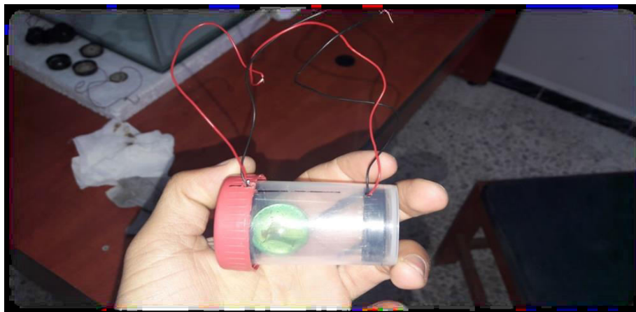
Figure 16: Glass balls placed inside the tube
