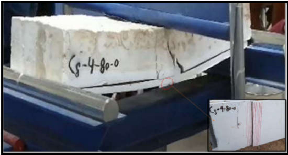
(c) Mode of failure for Cs-4-80-0 specimen.
