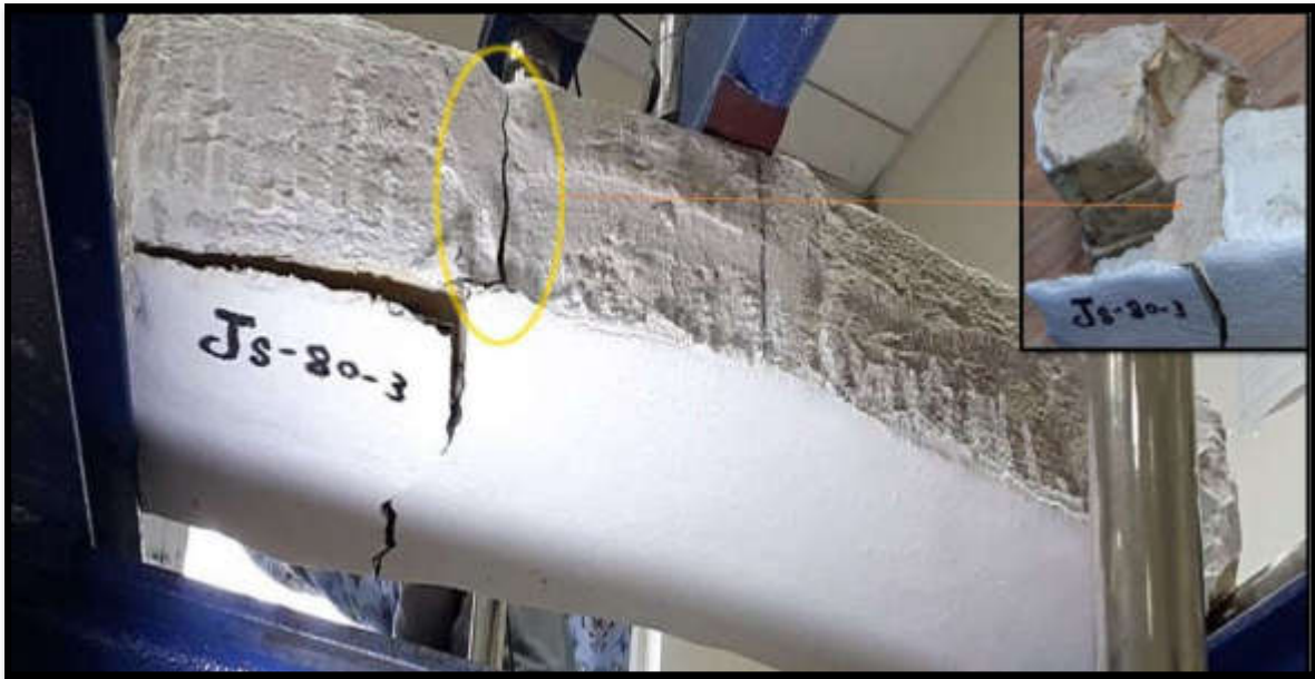
(c) Mode of failure for Js-80-3 specimen.
