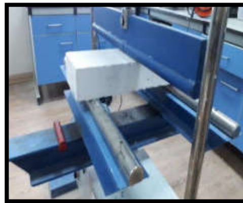
(e) Modulus of rupture test.
