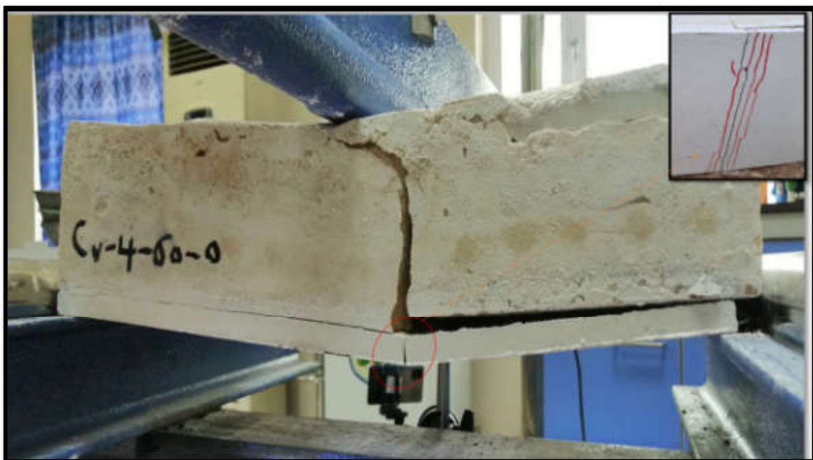
(h) Mode of failure for Cv-4-60-0 specimen.
