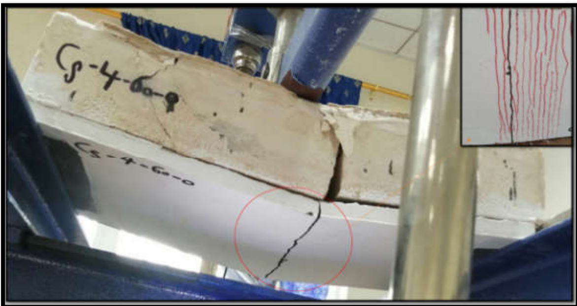
(b) Mode of failure for Cs-4-60-0 specimen.
