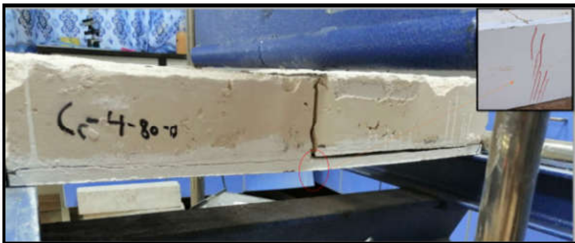
(k) Mode of failure for Cc-4-80-0 specimen.
