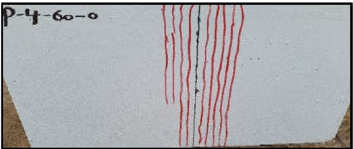
(b) Mode of failure for P-4-60-0 specimen.
