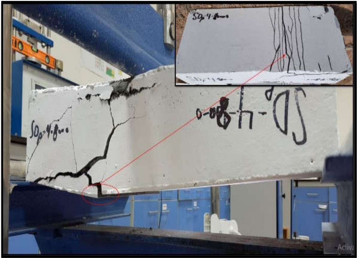
(g) Mode of failure for SDp-4-80-0 specimen.
