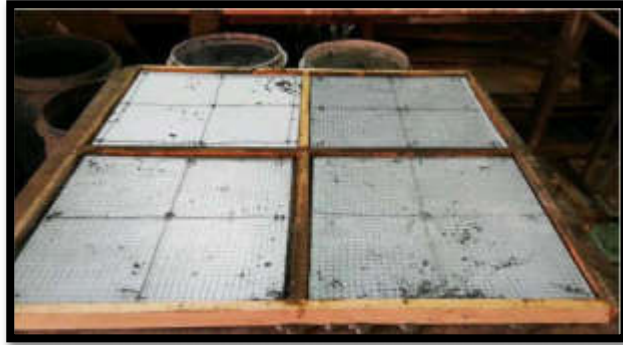
(b) fixing the reinforcement with core material.
