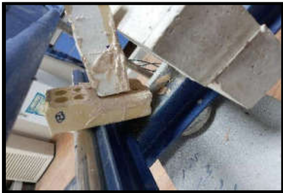
(c) Perforated clay bricks after failure.
