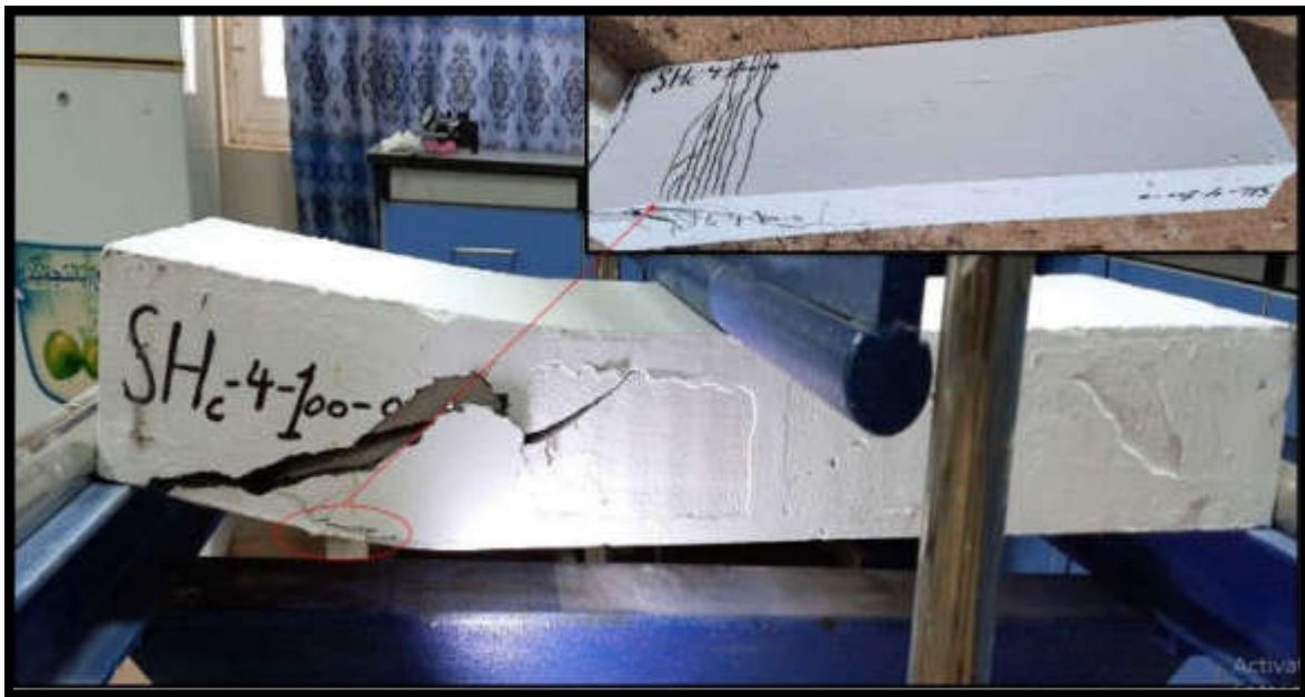
(e) Mode of failure for SHc-4-100-0 specimen.
