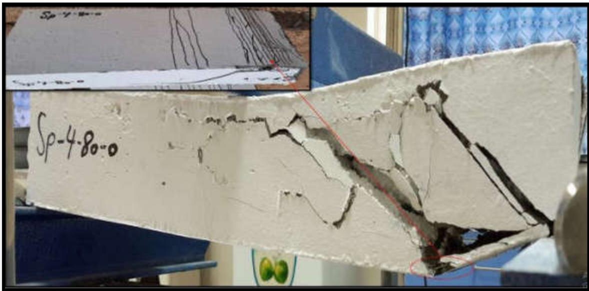
(c) Mode of failure for Sp-4-80-0 specimen.
