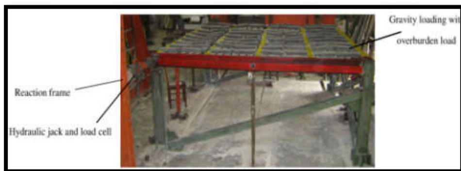
(a) Gravity loading detail.
