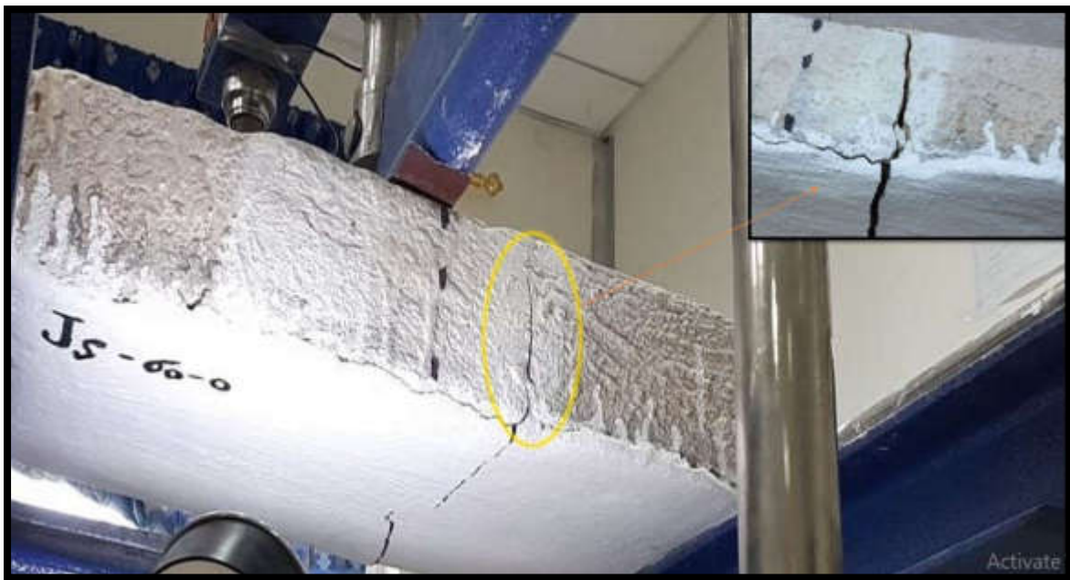
(a) Mode of failure for Js-60-0 specimen.
