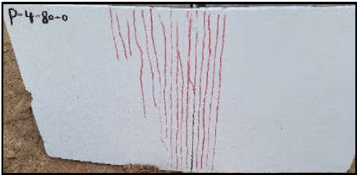
(c) Mode of failure for P-4-80-0 specimen.
