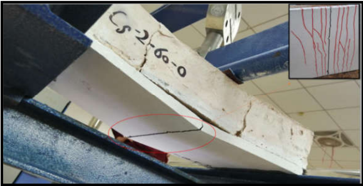
(a) Mode of failure for Cs-2-60-0 specimen.
