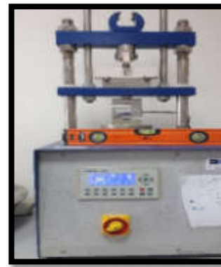
(e) Modulus of rupture test.
