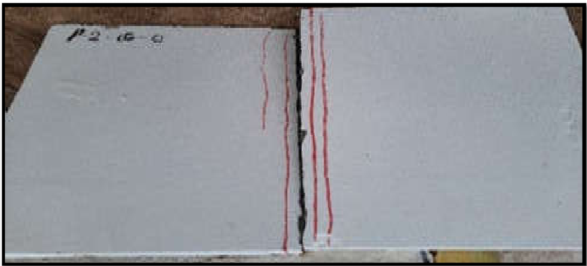
(a) Mode of failure for P-2-60-0 specimen.
