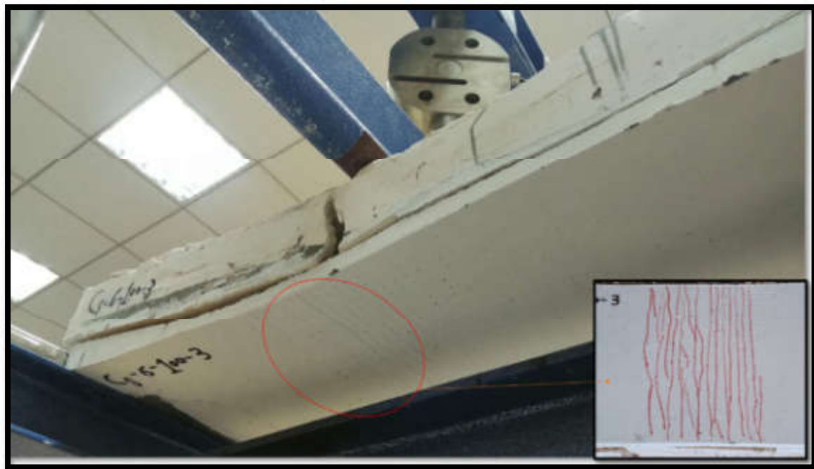
(g) Mode of failure for Cs-6-100-3 specimen.
