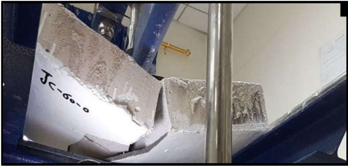
(e) Mode of failure for Jc-60-0 specimen.
