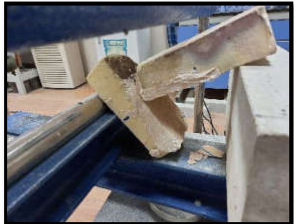
(b) Solid bricks after failure.
