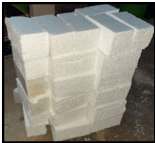
Figure. 3-6: Styropor prism of (200 ×100 ×100)mm.
