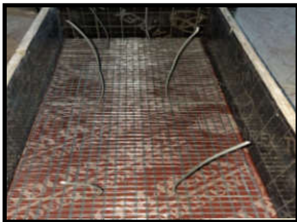
(c) Shear connectors at bottom.
