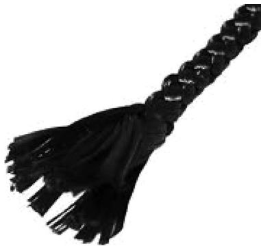
Fig. 3 Fiber-reinforced polymer rope (FRPR) sample
