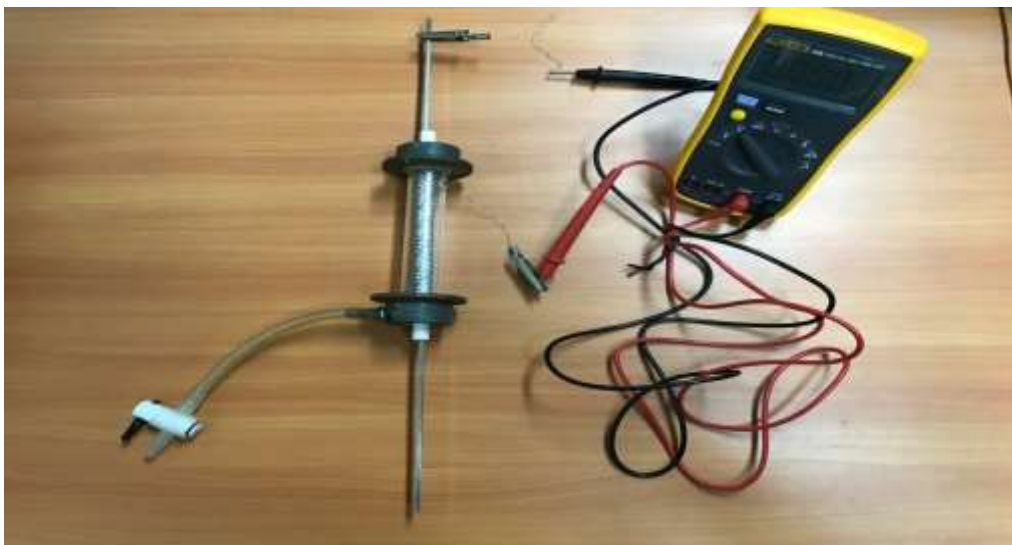
Figure 3.12 Represents the Basic Cell which Used in the Measurement of Zeta Potential, Consist of the Ceramic Membrane was Mounted in Transparent uPVC Module House, Outside Electrode and Inside Electrode were Connected to Nigh Impedance Milli-Voltmeter.
