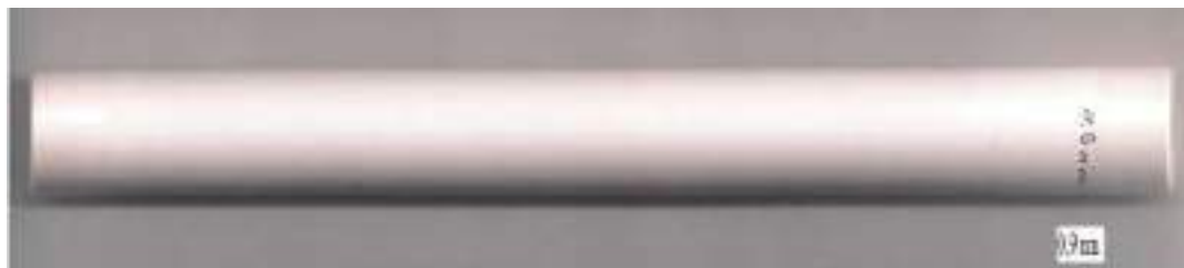
Figure 3.7 Vergin Ceramic Titanium Dioxide NF Membrane with Pore Size of 0.9 nm, Length = 19 cm, ID = 7 mm, OD = 10 mm.
