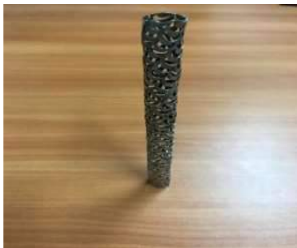
Figure 3.1 Represent the Outside Electrode form, it was Made from the (Silver and 4% Gold), Length = 14 cm, ID = 10.0 mm, OD = 10.4 mm.
