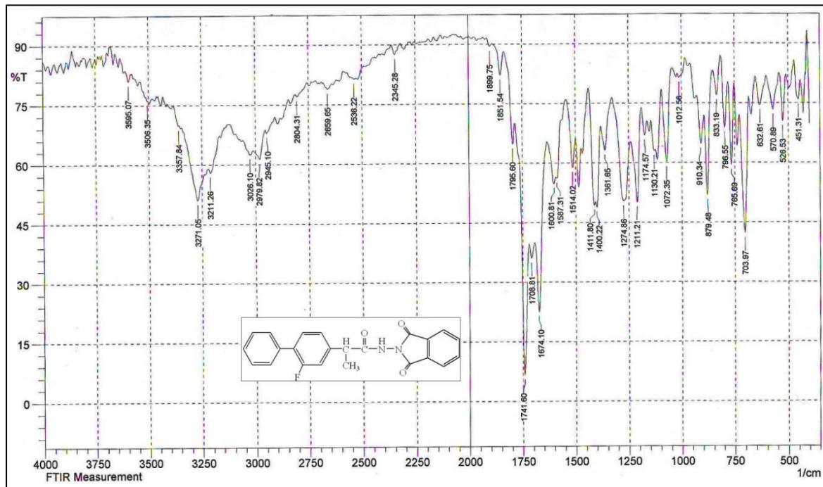
Figure (3.5): FT-IR spectrum of compound [5].
