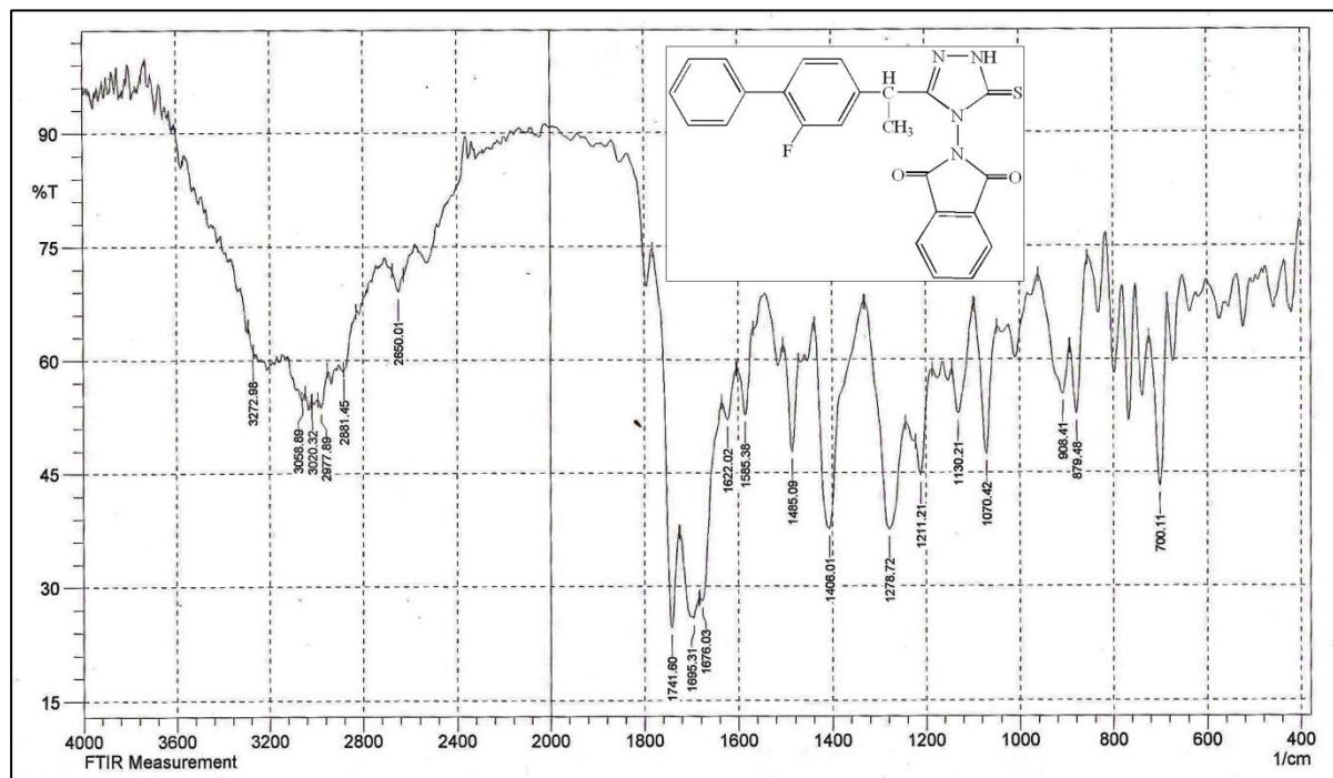
Figure (3.19): FT-IR spectrum of compound [13].
