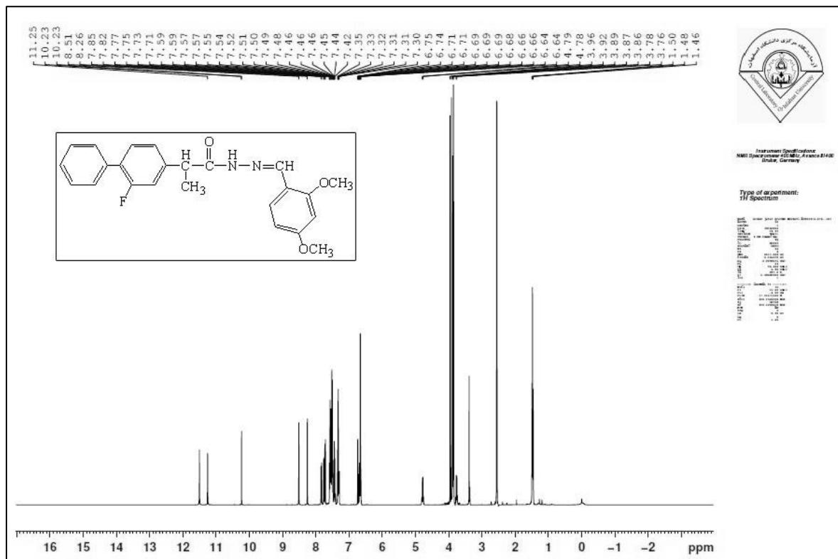
Figure (3.10):  $^1\text{H}$ -NMR spectrum of compound [6].
