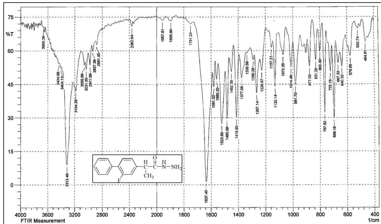
Figure (3.2): FT-IR spectrum of compound [2].
