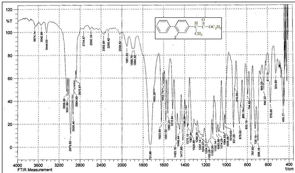
Figure (3.1): FT-IR spectrum of compound [1].
