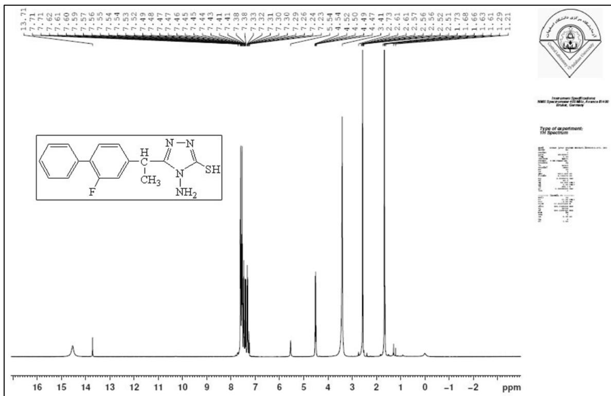
Figure (3.15):  $^1\text{H-NMR}$  spectrum of compound [10].
