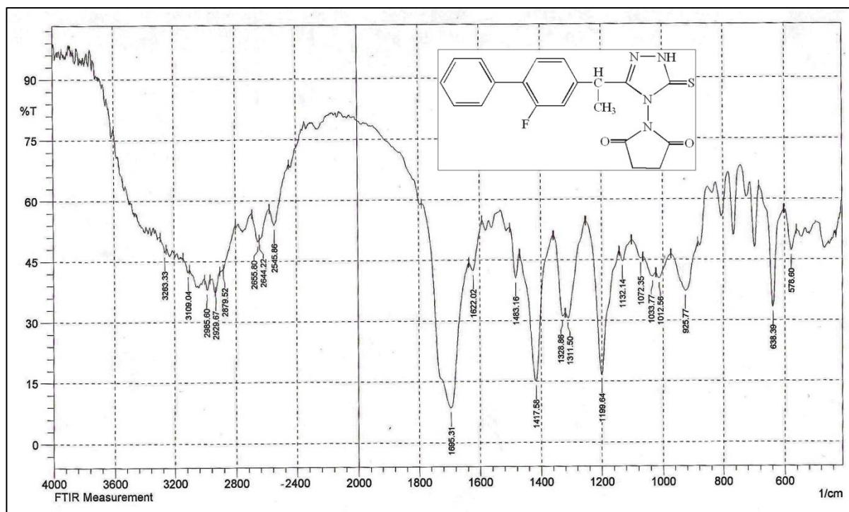
Figure (3.18): FT-IR spectrum of compound [12].
