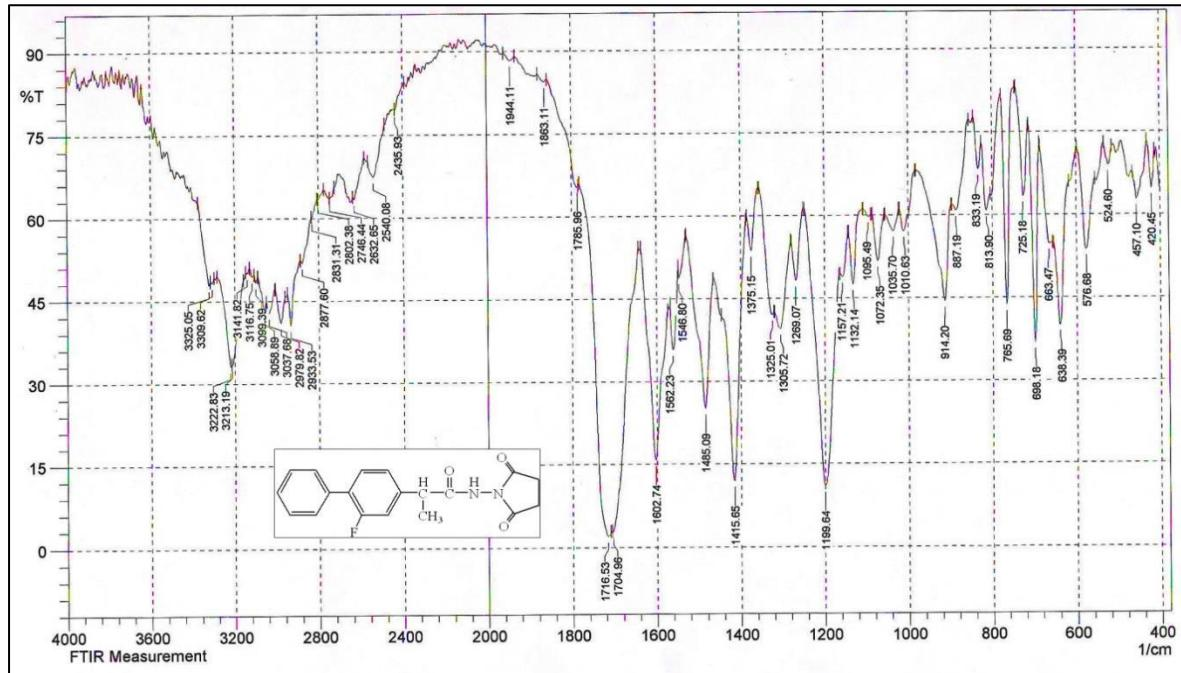
Figure (3.4): FT-IR spectrum of compound [4].
