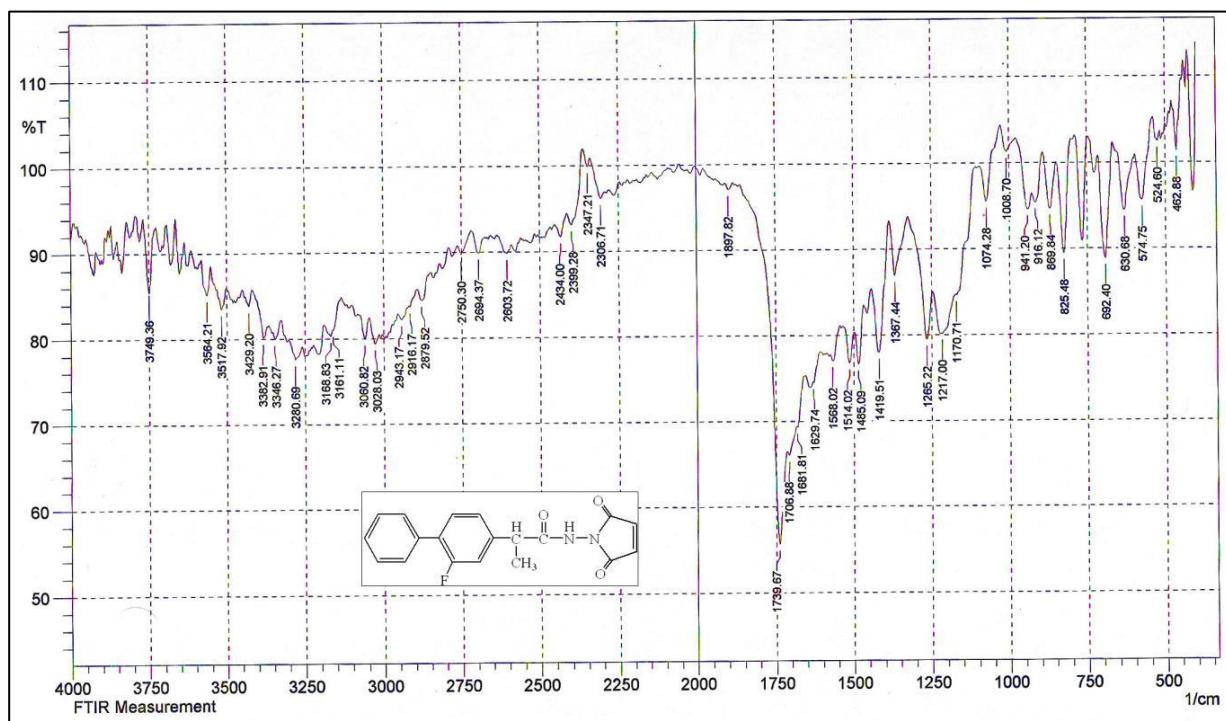
Figure (3.3): FT-IR spectrum of compound [3].
