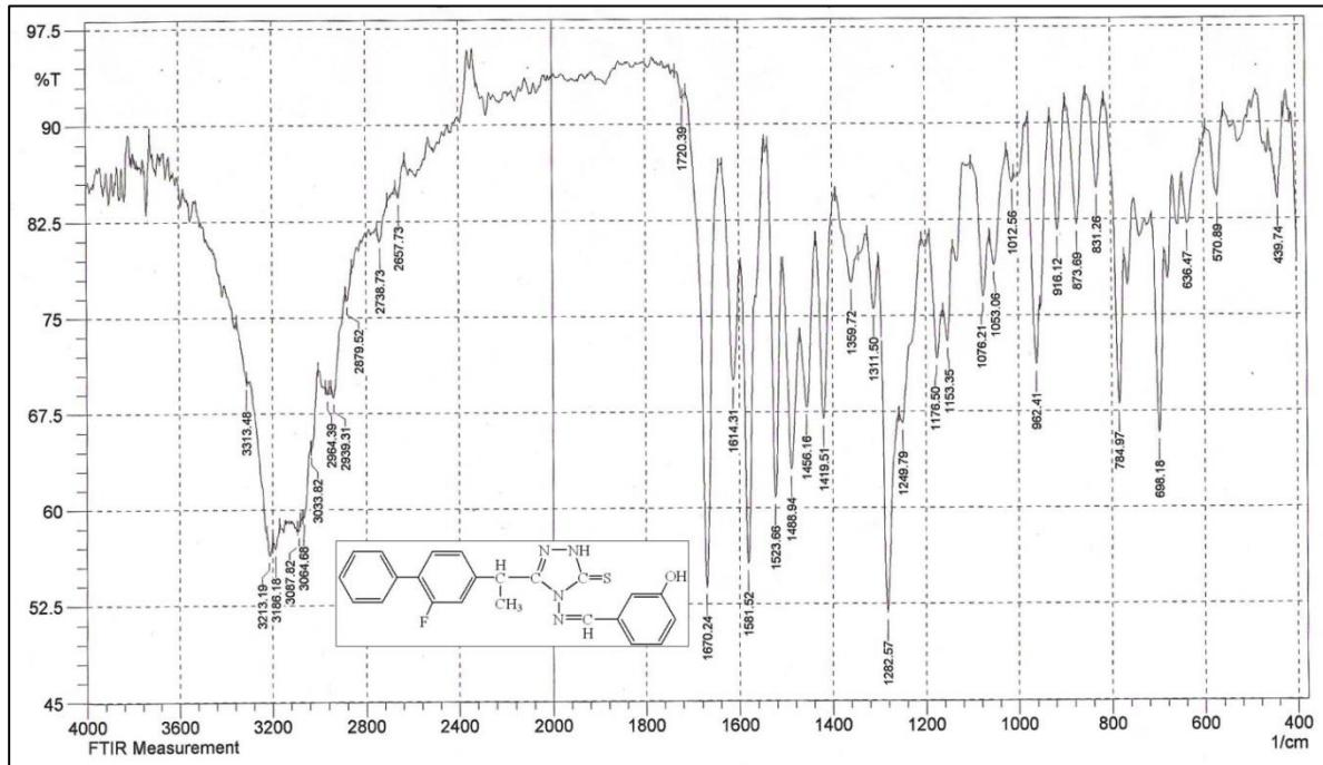
Figure (3.22): FT-IR spectrum of compound [16].
