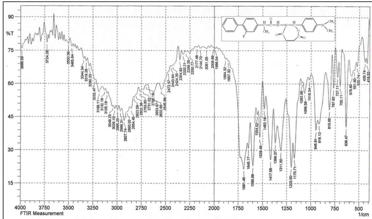
Figure (3.37): FT-IR spectrum of compound [27].
