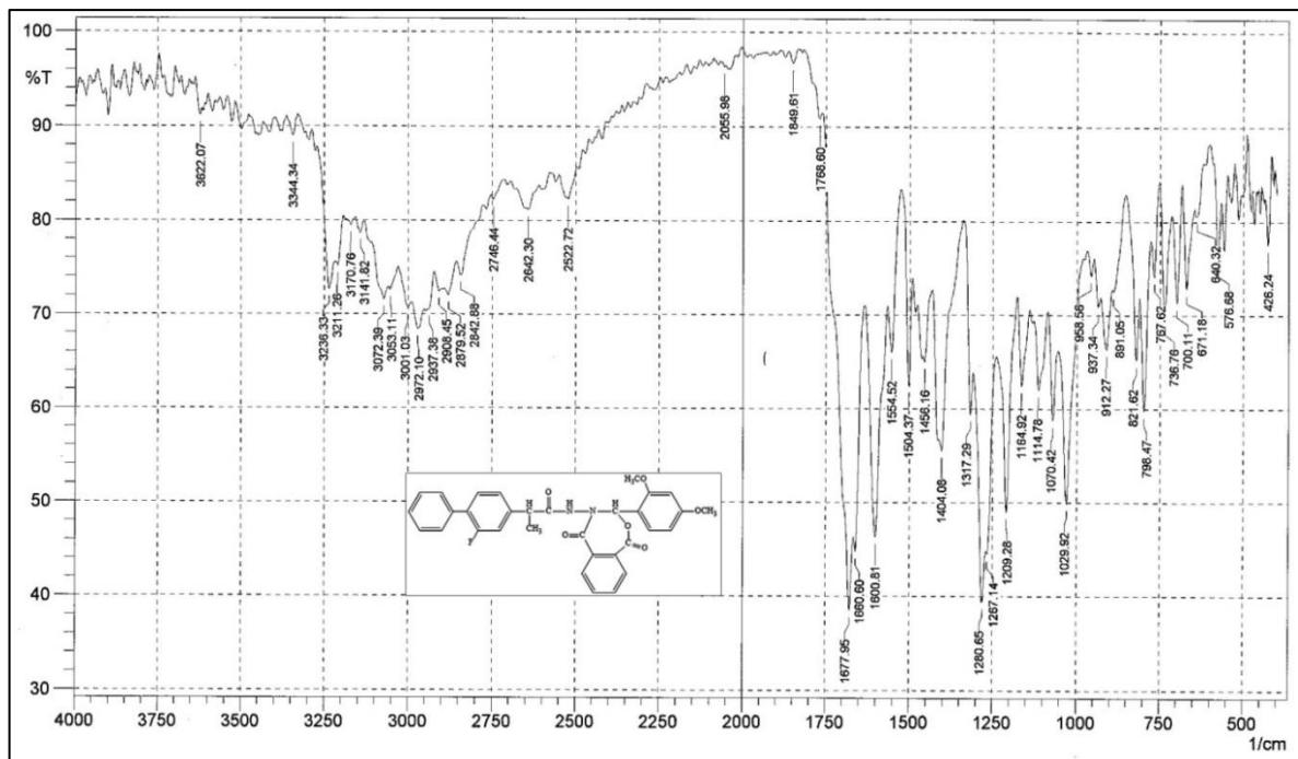
Figure (3.40): FT-IR spectrum of compound [30].
