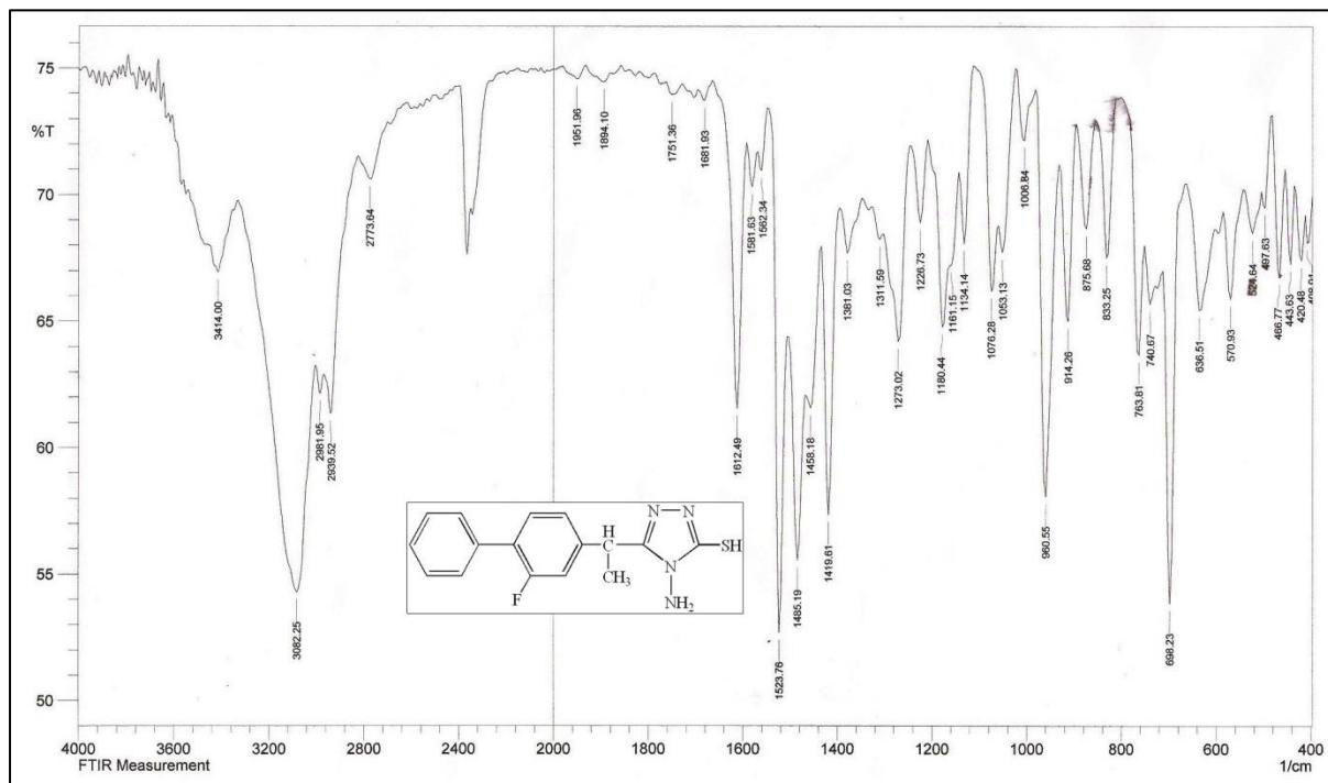
Figure (3.14): FT-IR spectrum of compound [10].
