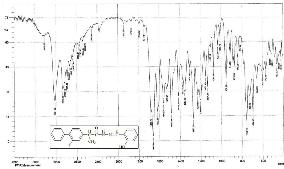
Figure (3.9): FT-IR spectrum of compound [9].
