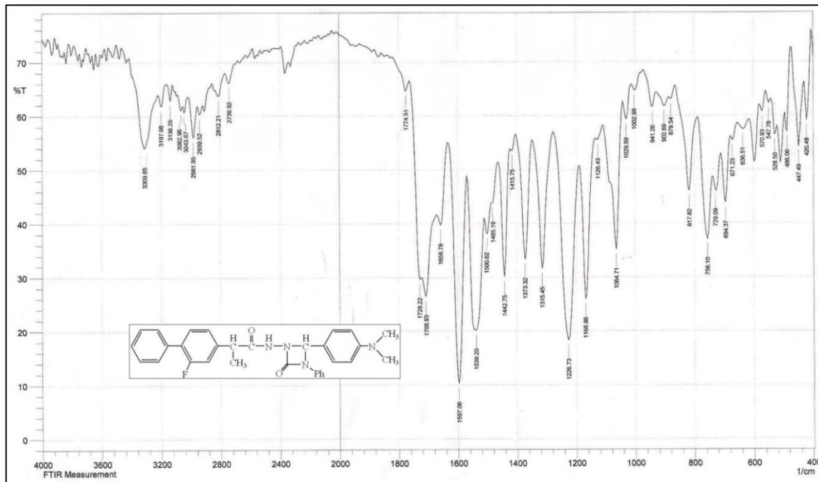
Figure (3.27): FT-IR spectrum of compound [19].
