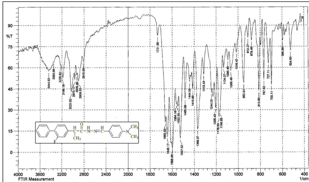
Figure (3.7): FT-IR spectrum of compound [7].
