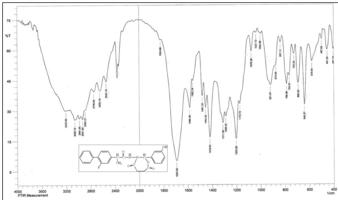
Figure (3.38): FT-IR spectrum of compound [28].
