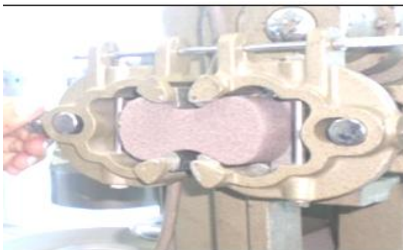
Figure 3. The sample was clamped between the attachments of the universal silica strength machine
