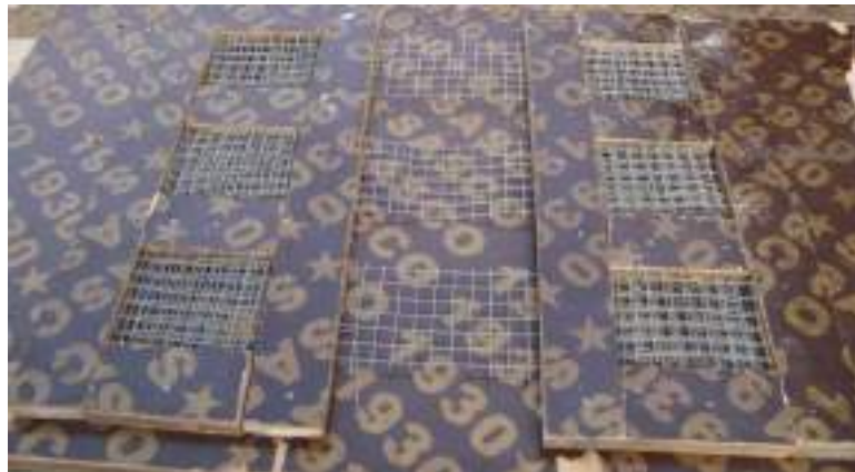
Plate (3.1) Tested WWM Coupon inserted in the wooden mold before applying mortar at ends
