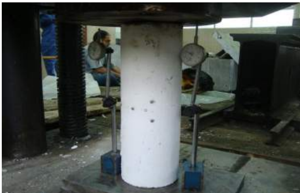
Plate (3.7) Test setup and instrumentation of tested columns
