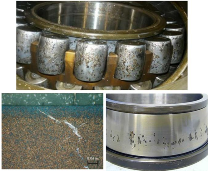
Figure 2. Examples of WECs found in WTGB [8][9]
