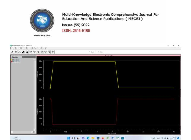
Figure (5). Input / output waveform of the NOT gate circuit
