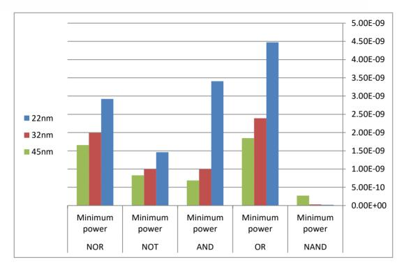
Figure (9). The minimum power of all gates with 22 nm, 32 nm, 45 nm techniques
