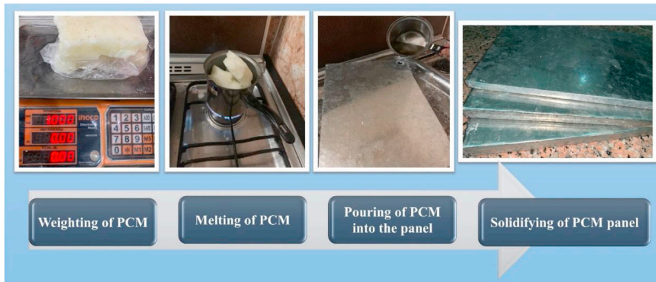
Fig. 3. Preparation of PCM panels.
