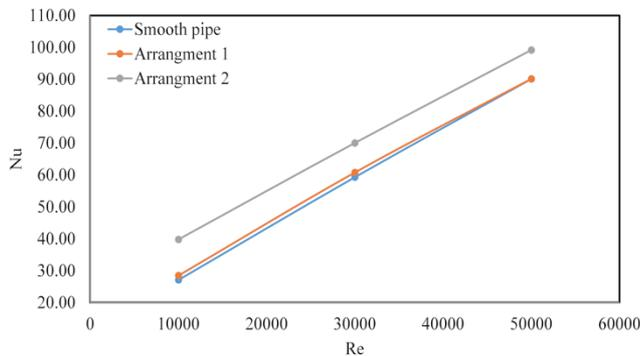
Fig. 6. The variation of the average  $Nu$  with  $Re$  for Smooth and baffled pipe.
