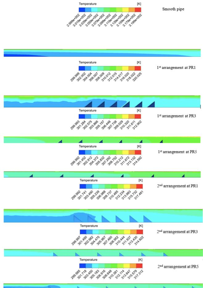
Fig. 14. Temperature distribution contour comparison of smooth pipe with baffled pipe at ( $Re=10000$ ).
