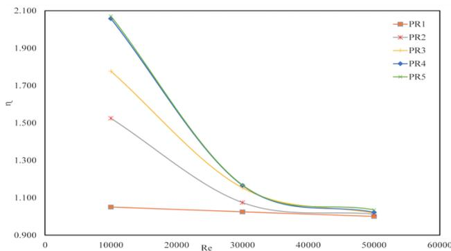
Fig. 12. Variations of Thermal Performance vs. Reynolds Numbers for the first arrangement at PR 1, 2, 3, 4 and 5.
