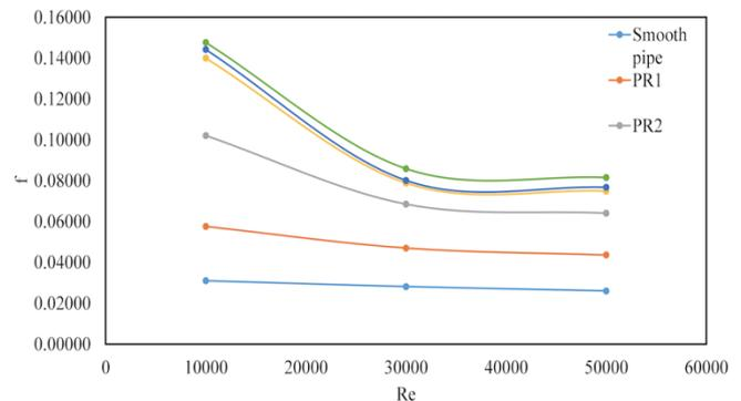
Fig. 10. Variations of friction factor vs. Reynolds Numbers for the first arrangement at PR 1,2,3,4 and 5.
