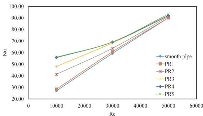
Fig. 8. Average  $Nu$  versus  $Re$  values for Smooth and baffled pipe (arrangement 1) for PR 1-5.
