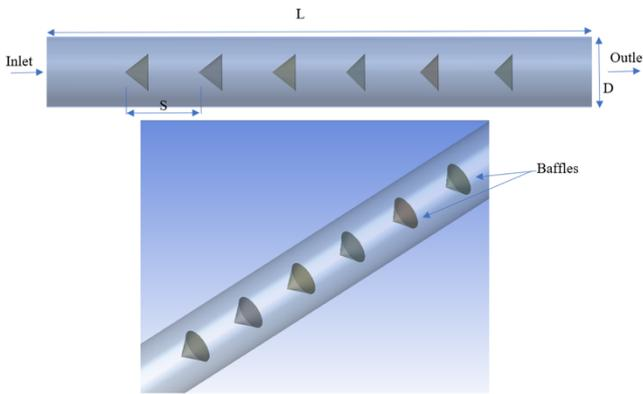
Fig. 1. 3D and side view of baffles inside the pipe.
