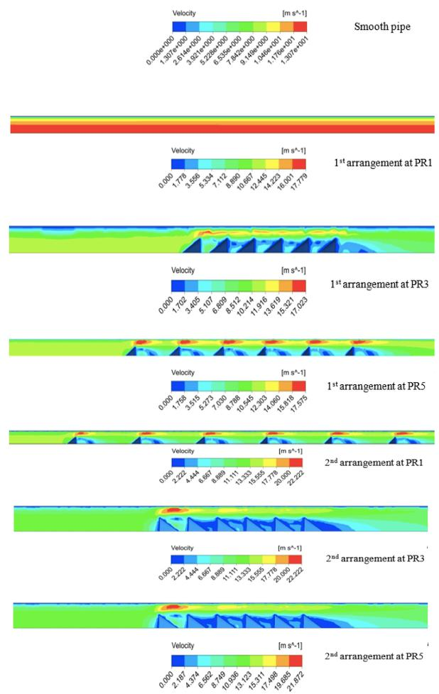
Fig. 4. Velocity distribution contour at ( $Re = 10000$ ) at PR (1,3,5) for both arrangements.
