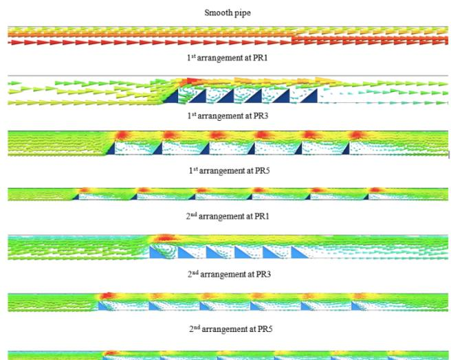
Fig. 5. Variation of swirl flow ( $Re = 10000$ ) at PR (1,3,5) at both arrangements.
