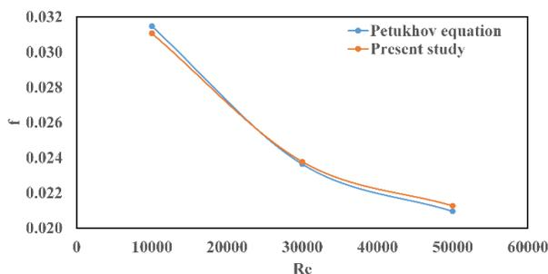
Fig. 3. The friction factor calculated in the present with Petukhov equation.
