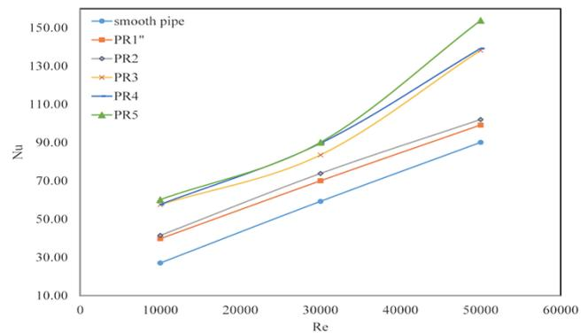
Fig. 9. Average  $Nu$  versus  $Re$  values for Smooth and baffled pipe (arrangement 2) for PR 1-5.
