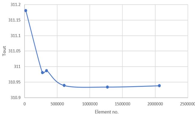
Fig. 2. outlet temperature VS mesh element number.
