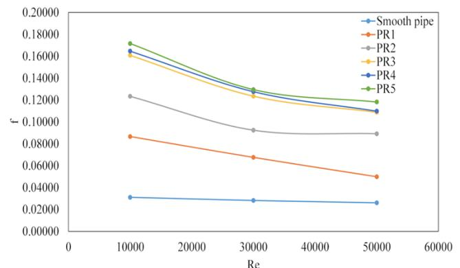
Fig. 11. Variations of friction factor vs. Reynolds Numbers for the second arrangement at PR 1, 2, 3, 4 and 5.
