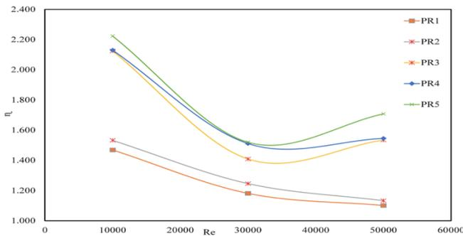
Fig. 13. Variations of Thermal Performance vs. Reynolds Numbers for the second arrangement at PR 1, 2, 3, 4 and 5.
