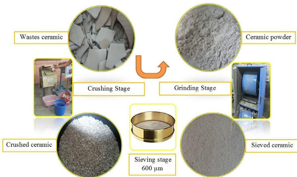
Fig. 1. Process of preparation of WCP in the lab.
