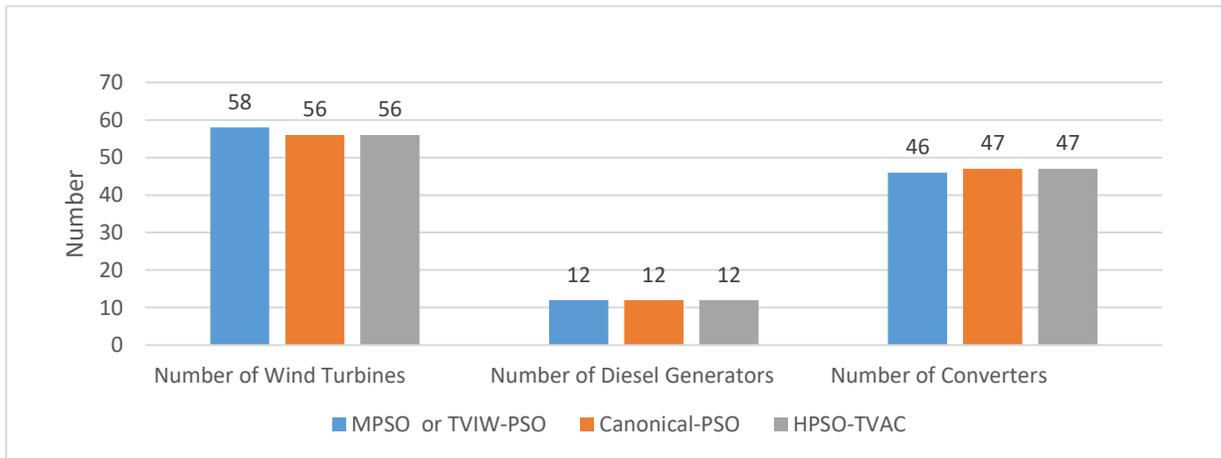
Figure 5. Comparison of the numbers of wind turbines, DG and converters obtained among types of PSO algorithm
