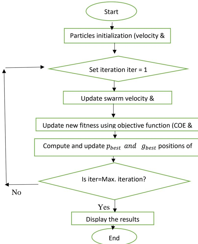
Figure 2. Flowchart of the PSO algorithm.
