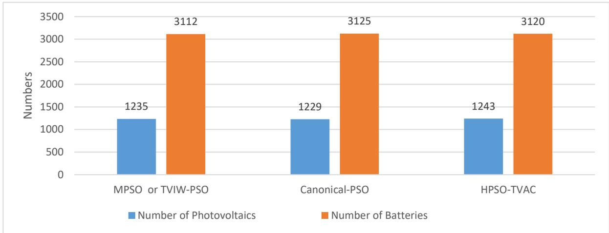
Figure 4. Comparison of the numbers of photovoltaics and bank batteries obtained among types of PSO algorithm
