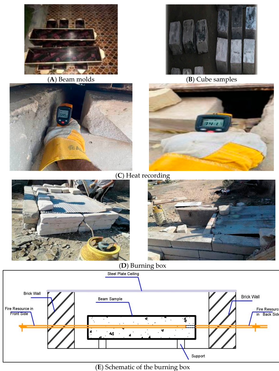
Figure 3. Testing and molds.
