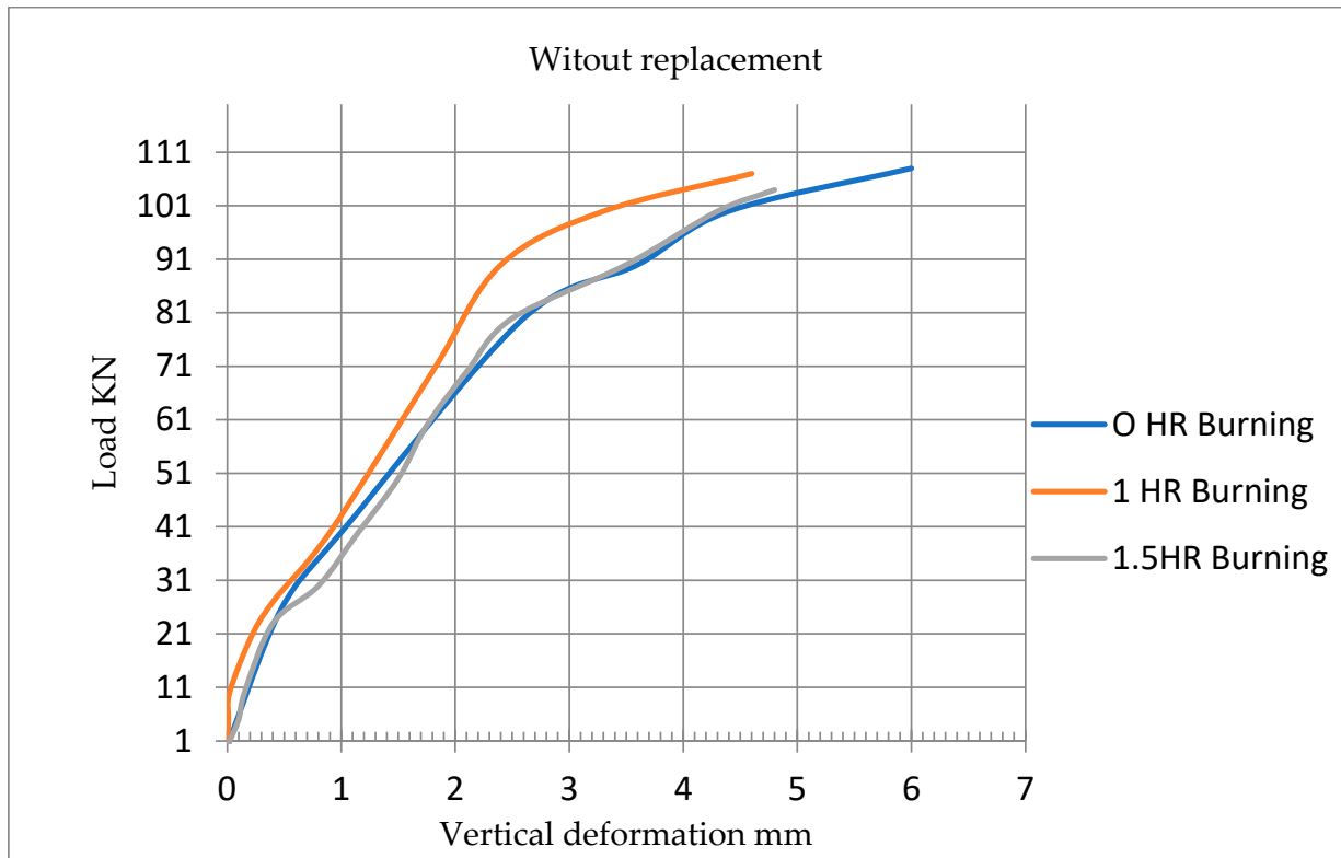
Figure 7. Load–deflection curves of beams without replacement.
