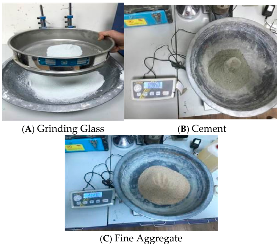
Figure 1. Samples of Grinding Glass, cement and fine aggregate.
