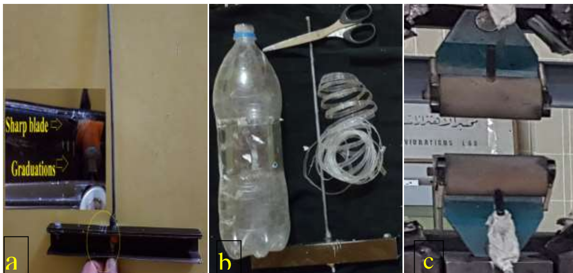
Fig.(2),a-PET bottle cutter tool, b- Cutting PET bottle method, c-Tensile testing of one PET strip.
