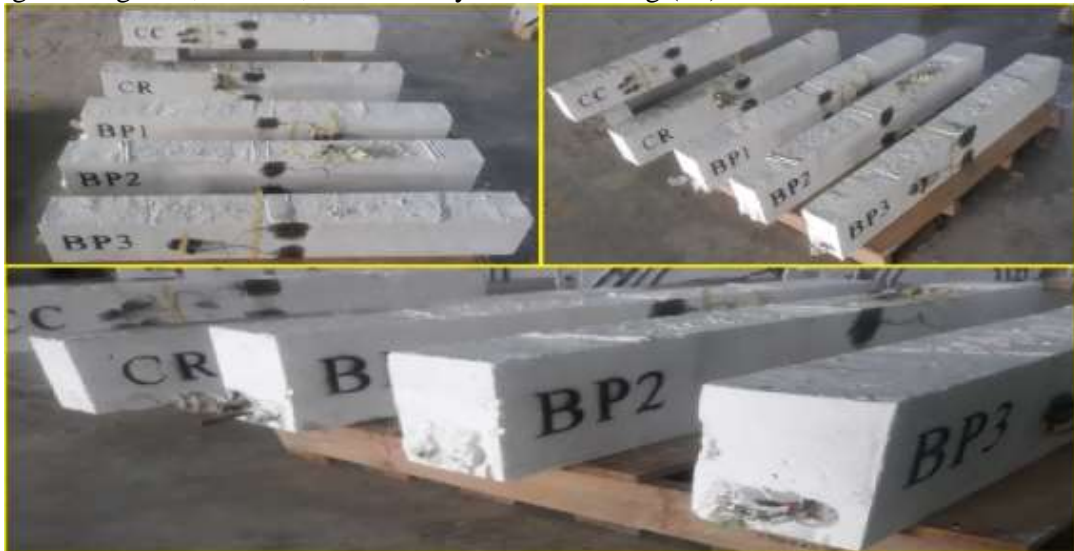
Fig. (10): Beam specimens for the part of replacing main reinforcement
