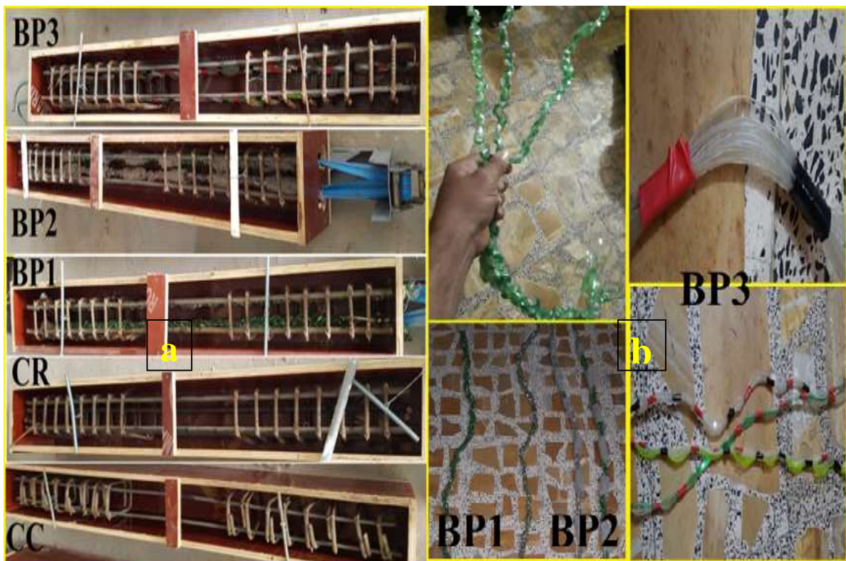
Fig. (4) a- Types of reinforcement for all concrete beams, b- type of PET waste bars
