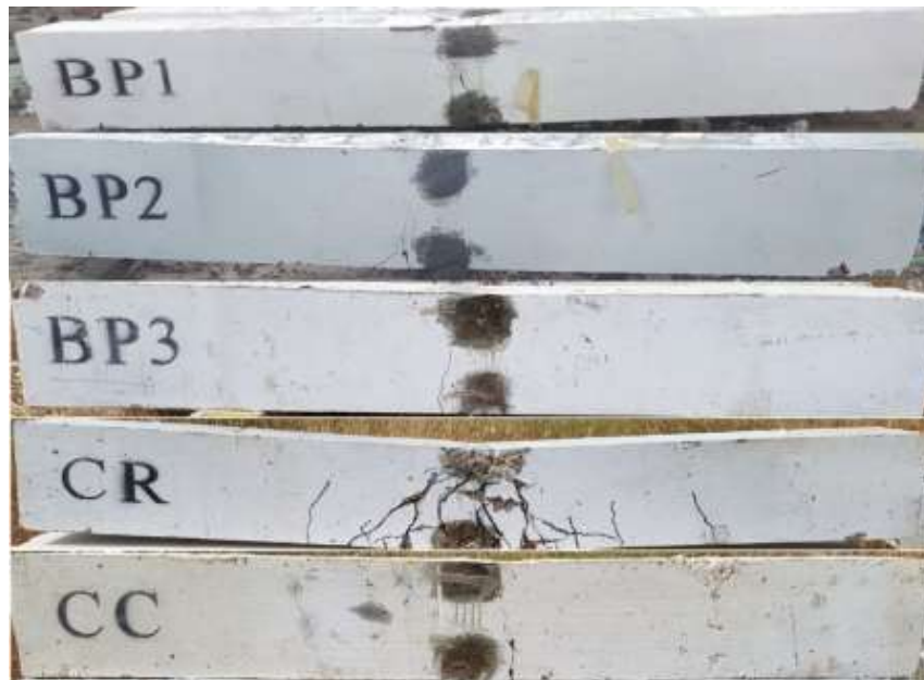
Fig. (17): Crack pattern of all beams specimens
