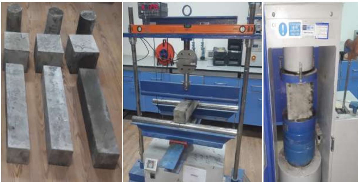
Fig.(9) Mechanical properties specimens and testing method
