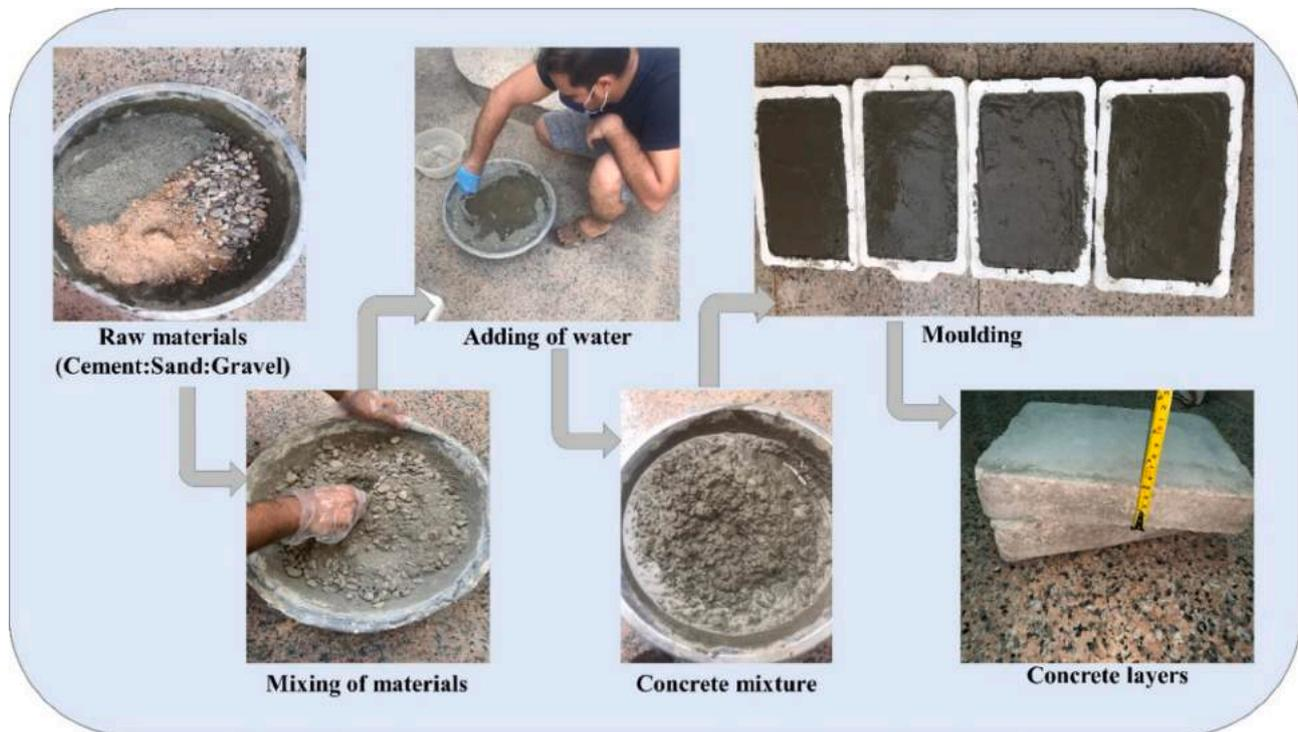
Fig. 2. Fabricating of concrete layers.
