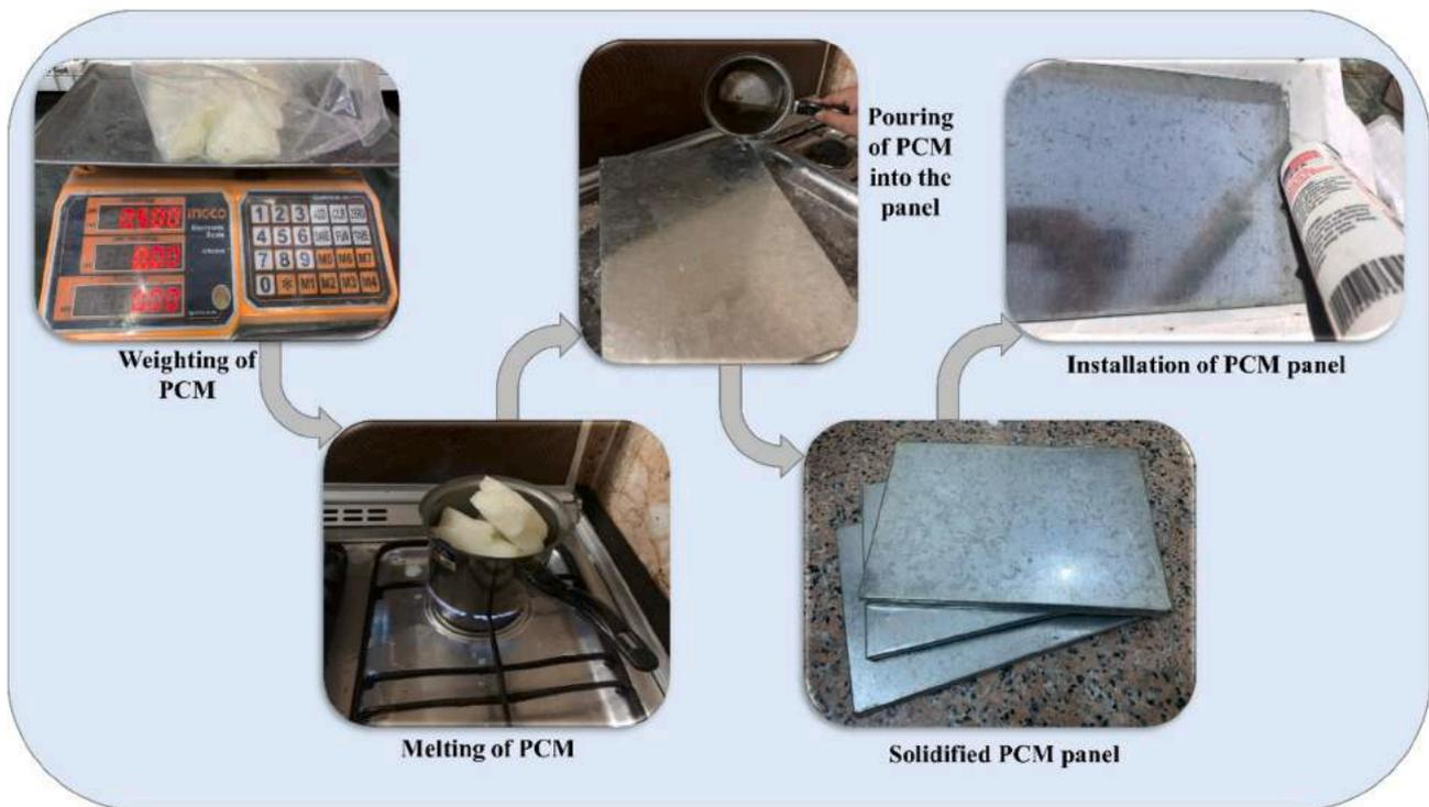
Fig. 3. Preparation of the PCM panel.
